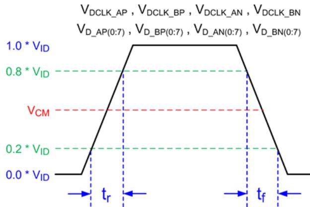
图 6-4. SubLVDS Input Rise and Fall Slew Rate
