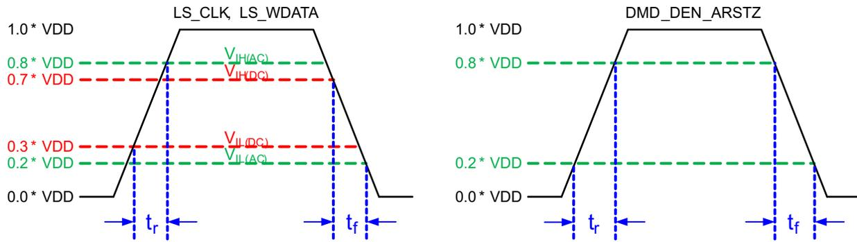
图 6-3. LPSDR Input Rise and Fall Slew Rate
