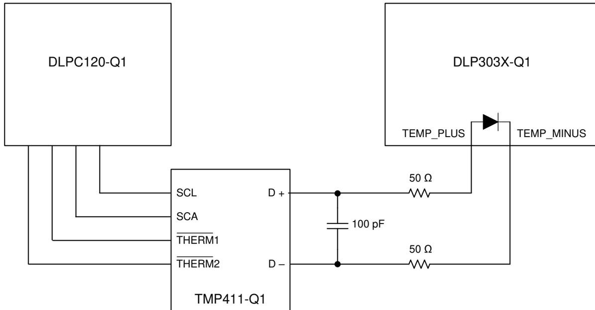
Figure 10. Temperature Sense Diode Typical Circuit Configuration
