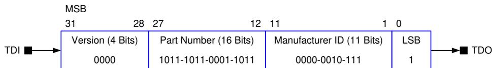
**Figure 14. DMD Device ID and 32-bit Shift Order**
