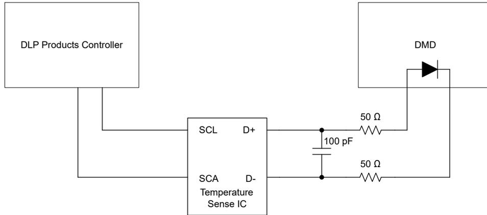
Figure 7-1. Temperature Sense Diode Typical Circuit Configuration
