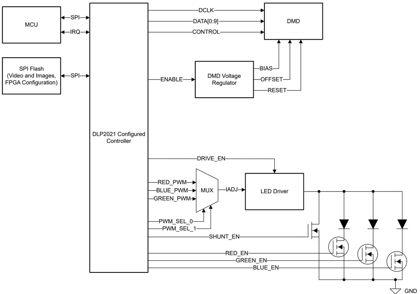
**図 8-1. Dynamic Ground Projection System Block Diagram**
