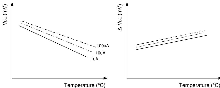
Figure 7-3. Example of Delta VBE vs. Temperature
