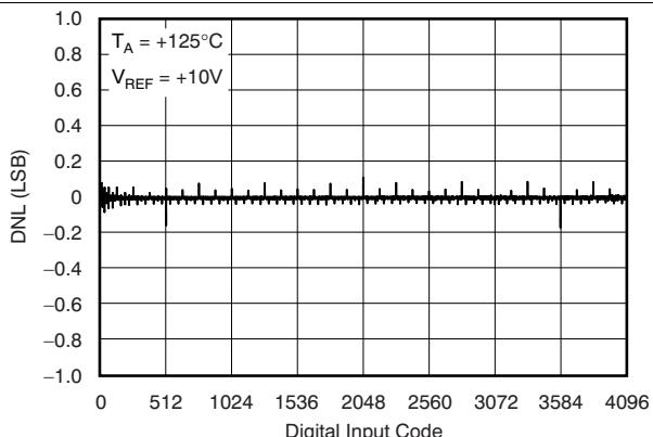
Figure 6. Differential Linearity Error vs Digital Input Code
