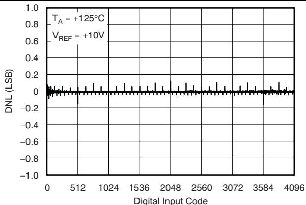
**Figure 20. Differential Linearity Error vs Digital Input Code**
