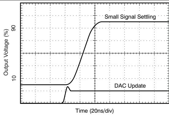
**Figure 11. DAC Settling Time**
