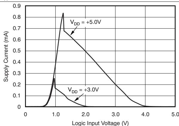
**Figure 7. Supply Current vs Logic Input Voltage**
