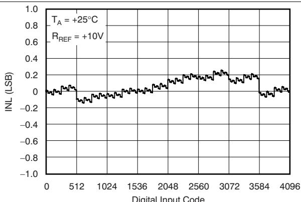
**Figure 15. Linearity Error vs Digital Input Code**
