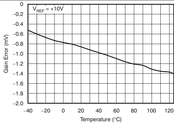
**Figure 12. Gain Error vs Temperature**
