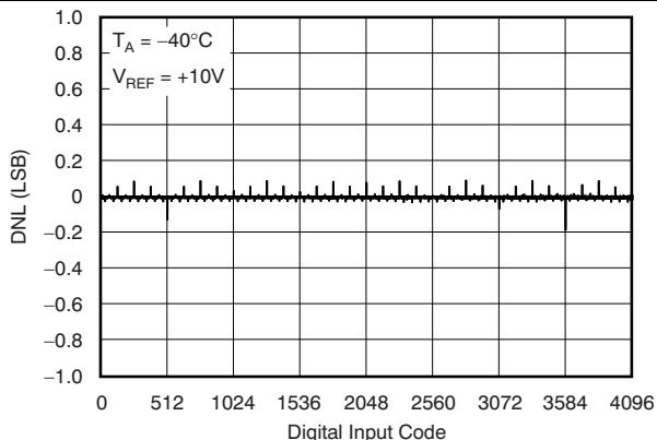
**Figure 18. Differential Linearity Error vs Digital Input Code**
