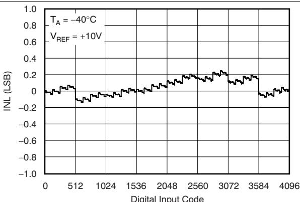
Figure 3. Linearity Error vs Digital Input Code
