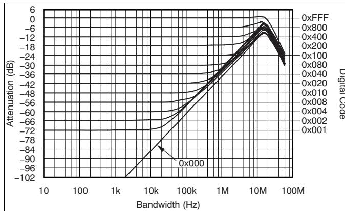
**Figure 8. Reference Multiplying Bandwidth**
