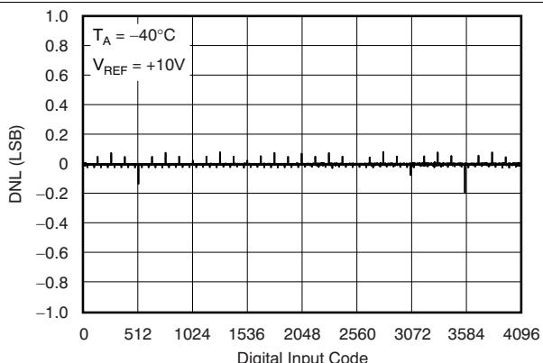
Figure 4. Differential Linearity Error vs Digital Input Code
