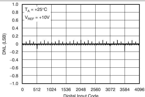
**Figure 16. Differential Linearity Error vs Digital Input Code**
