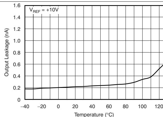
Figure 14. Output Leakage vs Temperature
