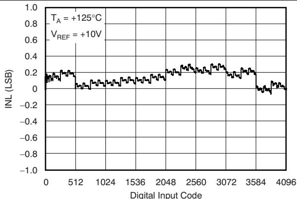
**Figure 19. Linearity Error vs Digital Input Code**
