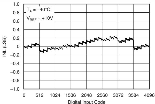
**Figure 17. Linearity Error vs Digital Input Code**
