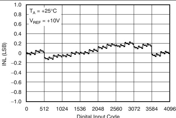
Figure 1. Linearity Error vs Digital Input Code
