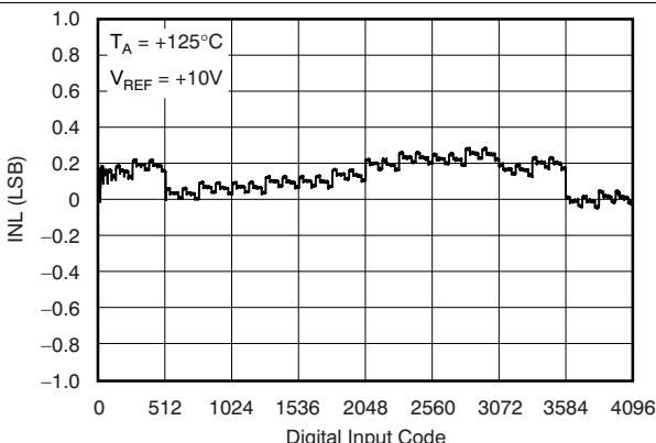
Figure 5. Linearity Error vs Digital Input Code
