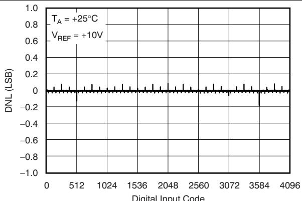
Figure 2. Differential Linearity Error vs Digital Input Code
