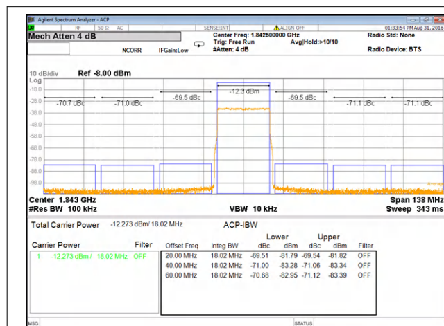
図 8-4. Dual band ACPR Performance in Downlink Band 3 with On-chip PLL
