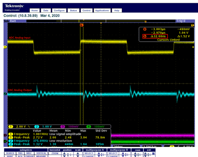
Figure 8-4. ADC Input to DAC Output Time for MSB loopback test.
