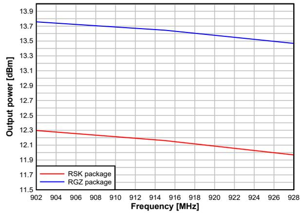
**7-18. Output Power vs. Frequency (50kbps, 915MHz, +14dBm)**
