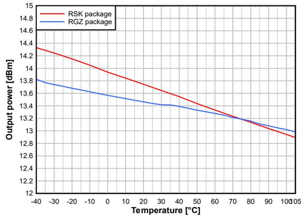
**7-15. Output Power vs. Temperature (50kbps, 868.3MHz, +14dBm)**
