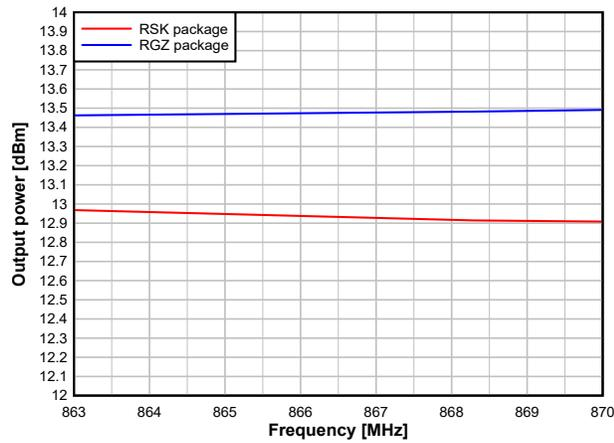
**7-17. Output Power vs. Frequency (50kbps, 868MHz, +14dBm)**
