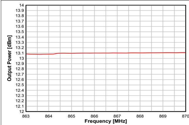
8-21. Output Power vs. Frequency (+14 dBm setting)
