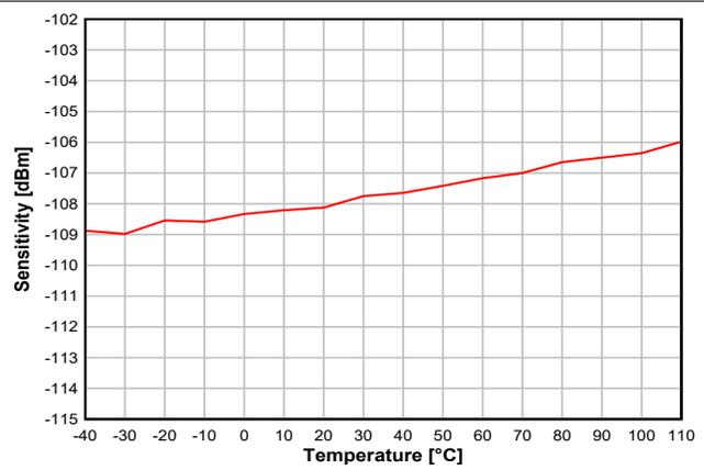
8-13. Sensitivity vs. Temperature (50 kbps, 868.3 MHz)
