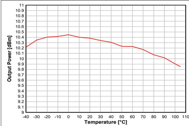
8-19. Output Power vs. Temperature (868.3 MHz, +10 dBm setting)
