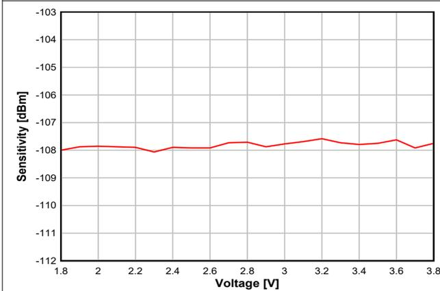
8-14. Sensitivity vs. Supply Voltage (VDDS) (50 kbps, 868.3 MHz)
