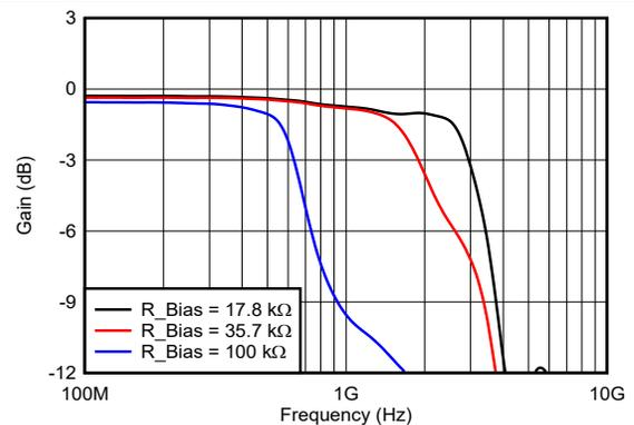
**6-6. Frequency Response vs  $R_{\text{Bias}}$  Resistance**
