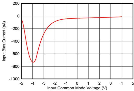
**6-25. Input Bias Current vs Input Common Mode Voltage**
