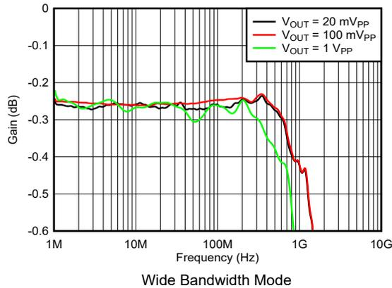
**6-3. Frequency Response vs Output Voltage, 0.1 dB Flatness**
