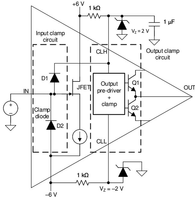
**FIG 8-2. Internal Input and Output Over-Voltage Clamp**
