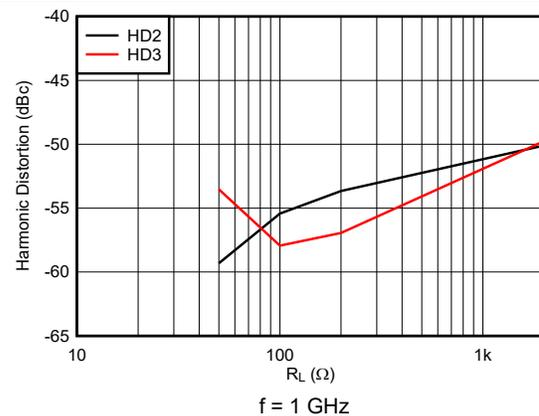
Figure 6-18. Harmonic Distortion vs Output Load
