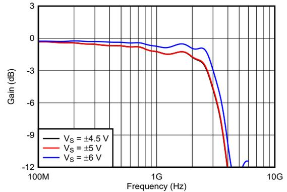
**6-4. Frequency Response vs Supply Voltage**
