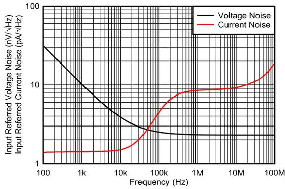
**6-19. Voltage and Current Noise Density vs Frequency**
