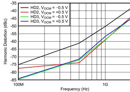
Figure 6-16. Harmonic Distortion vs Output Common Mode Voltage
