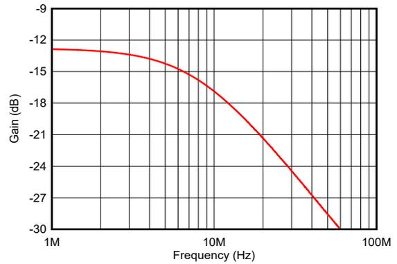
With RC pole of 2 kΩ and 10 pF at IN\_Aux pin
