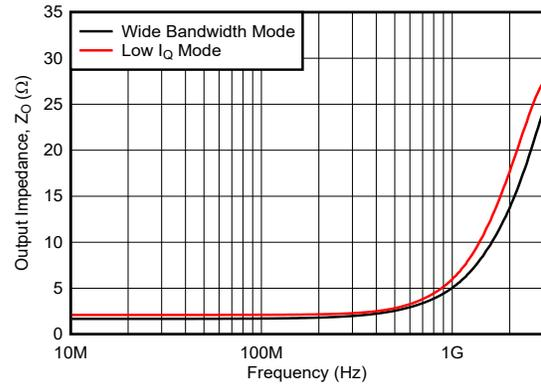
**6-22. Output Impedance vs Frequency**
