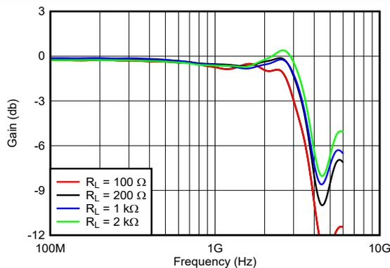
**6-5. Frequency Response vs Output Load**
