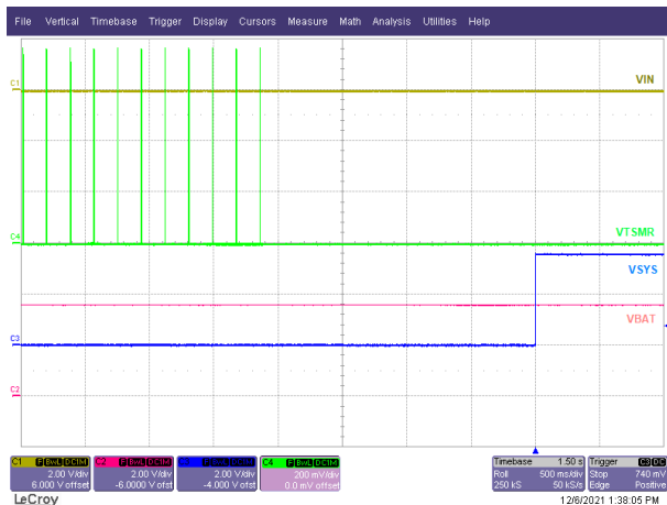
9-3. Power Up from Shutdown Mode with VIN Supply Insertion
