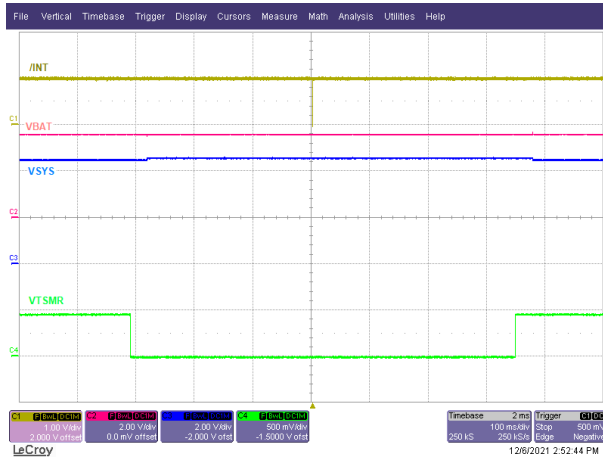
Figure 9-15. Wake1 Interrupt with VIN Present
