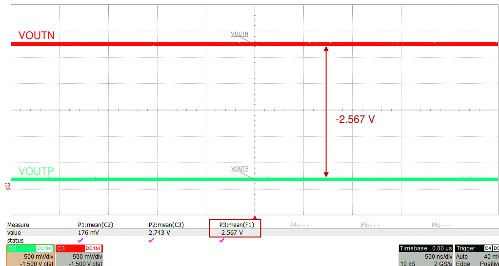
Figure 7-4. Typical Fail-Safe Output of the AMC3311-Q1
