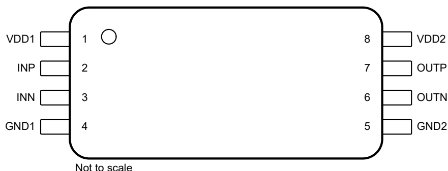
图 5-1. DWL Package, 8-Pin SOIC (Top View)
