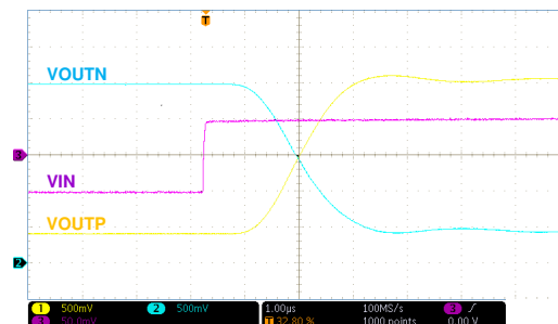
Figure 8-4. Step Response of the AMC1202
