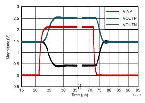
Figure 8-4. Step Response of the AMC0x11D
