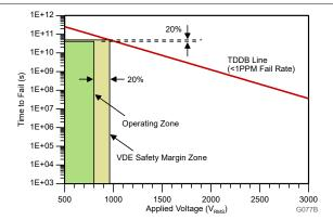
T<sub>A</sub> up to 150°C, stress-voltage frequency = 60Hz, isolation working voltage = 800V<sub>RMS</sub>, projected operating lifetime >>100 years
