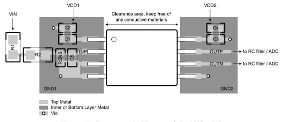
Figure 8-6. Recommended Layout of the AMC0x11D
