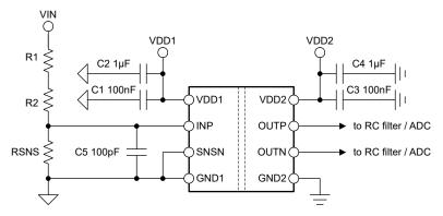
Figure 8-5. Decoupling of the AMC0x11D
