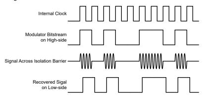
Figure 7-1. OOK-Based Modulation Scheme
