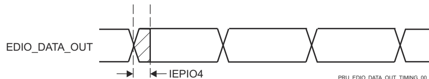
図 6-100. PRU_ICSSG IEP Digital IOs Timing Requirements
