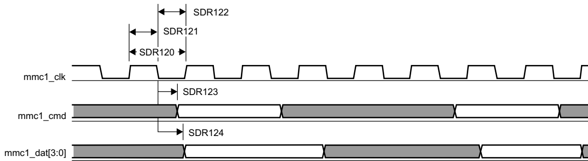
图 7-65. MMC/SD/SDIO in - High Speed SDR12 - Transmitter Mode
