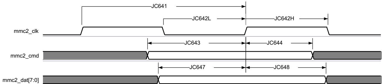
图 7-76. MMC/SD/SDIO in - High Speed JC64 - Receiver Mode
