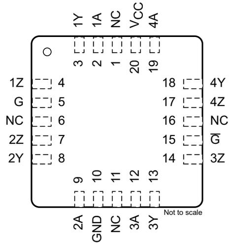
図 4-2. FK (LCCC) Package, 20-Pin (Top View)
