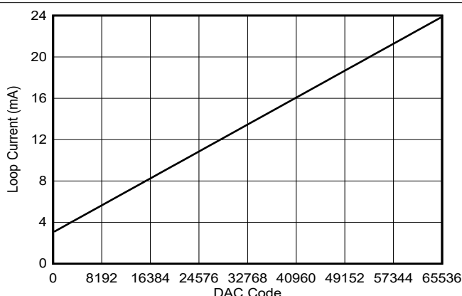
図 8-6. DAC Code to Loop Current
