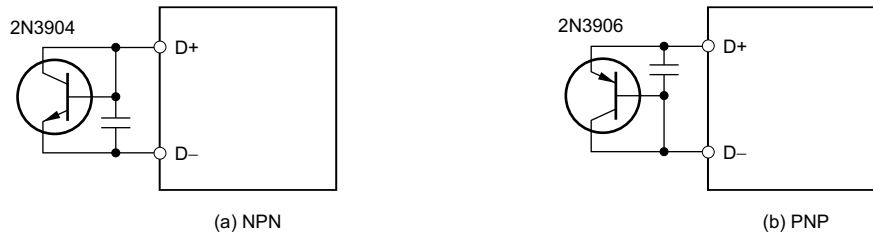
図 7-6. Remote Temperature Sensor Using Transistor
