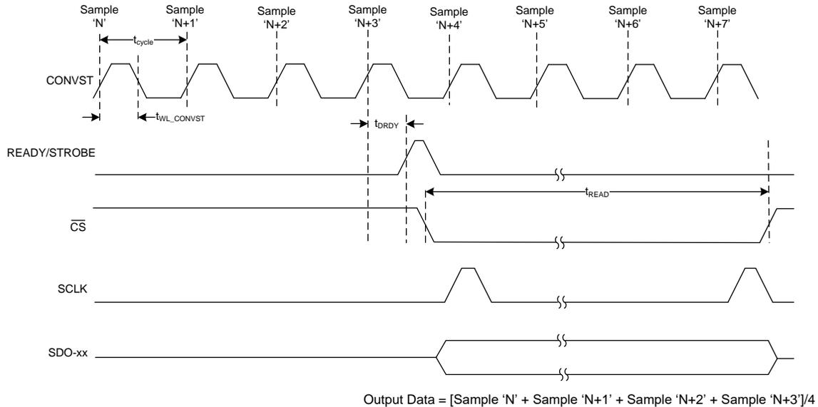
**Figure 42. Timing for Averaging of Four Samples**
