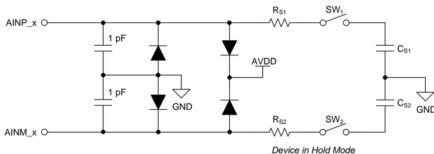
Figure 37. Analog Input Structure for Converter Module
