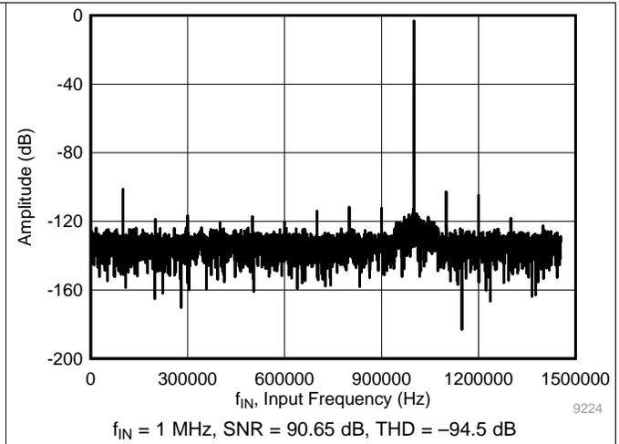
Figure 8. Typical FFT at  $f_{IN} = 1$  MHz
