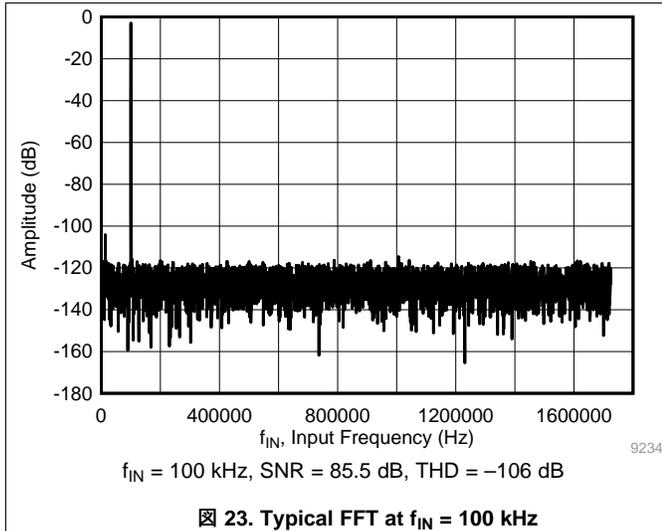
Figure 23. Typical FFT at  $f_{IN} = 100 \text{ kHz}$
