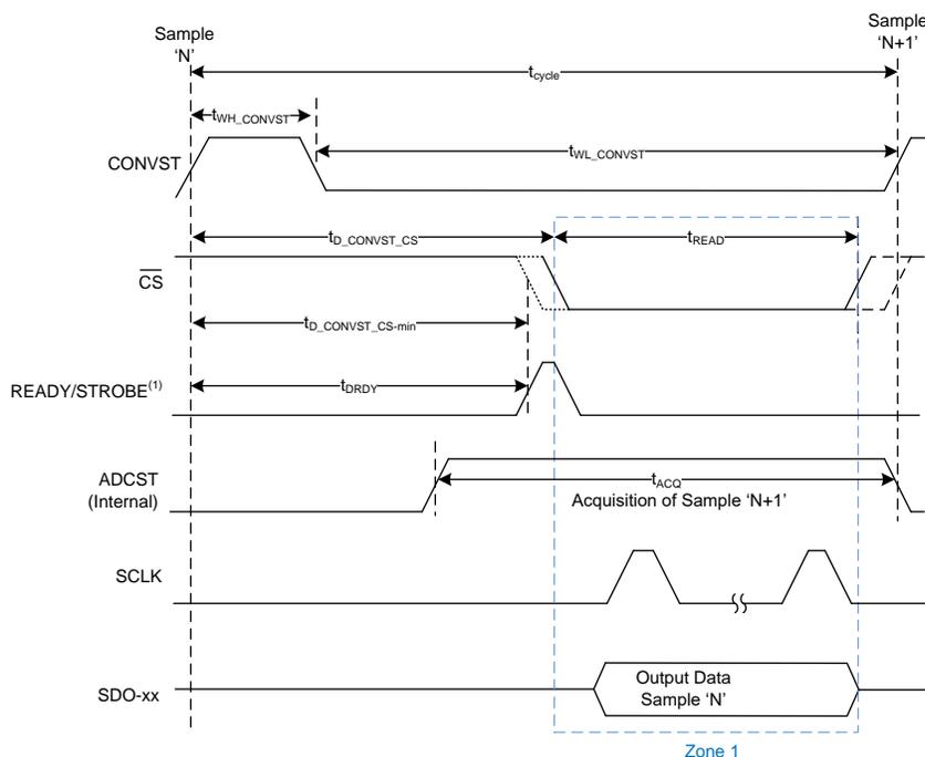
(1) The READY output is required for data transfer with zero cycle latency. The STROBE output is required only for clock re-timer (CRT) protocols.
