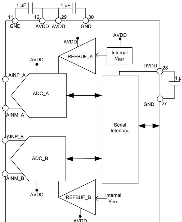
**Figure 83. Power-Supply Decoupling**
