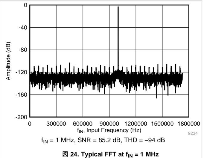
Figure 24. Typical FFT at  $f_{IN} = 1 \text{ MHz}$
