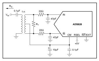
FIGURE 5. Transformer Coupled Input.
