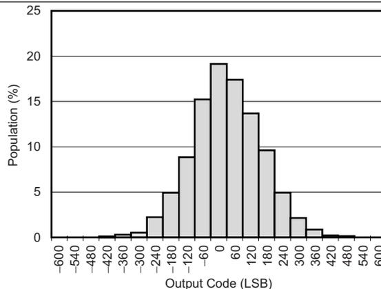
Gain = 64, data rate = 30 kSPS, buffer = off, 4096 readings
