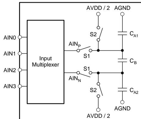
**Figure 25. Simplified Input Structure with Buffer Off**
