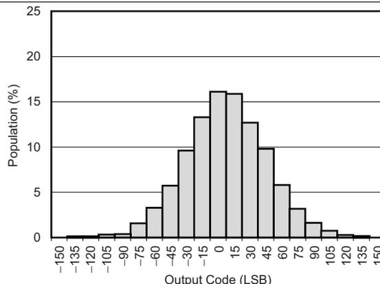
Gain = 64, data rate = 1 kSPS, buffer = off, 4096 readings
