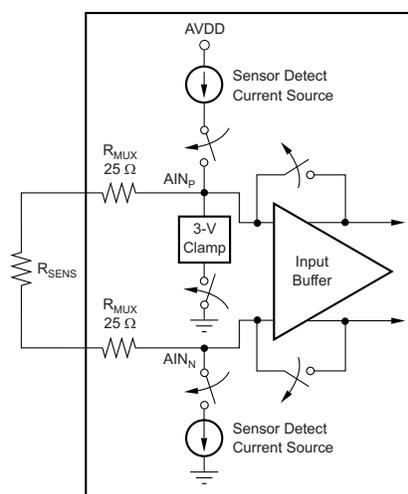
NOTE: Arrows indicate switch positions when the SDCS are enabled.
