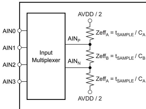
Figure 27. Analog Input Effective Impedances with Buffer Off
