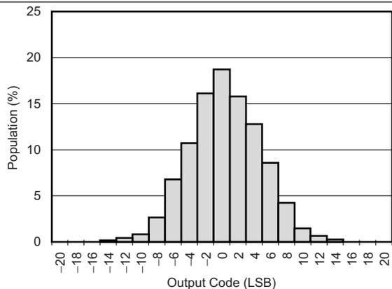
Gain = 1, data rate = 1 kSPS, buffer = off, 4096 readings
