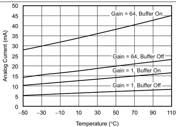
Figure 21. Analog Supply Current vs Temperature
