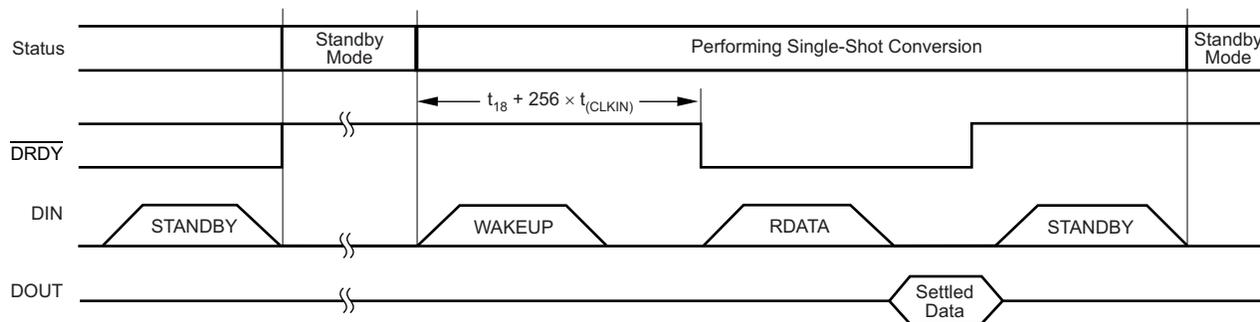
Figure 36. Single-shot Conversions Using the STANDBY Command
