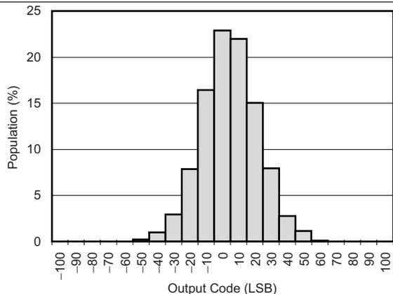
Gain = 1, data rate = 30 kSPS, buffer = off, 4096 readings
