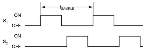
**Figure 26. S1 and S2 Switch Timing for Figure 25**
