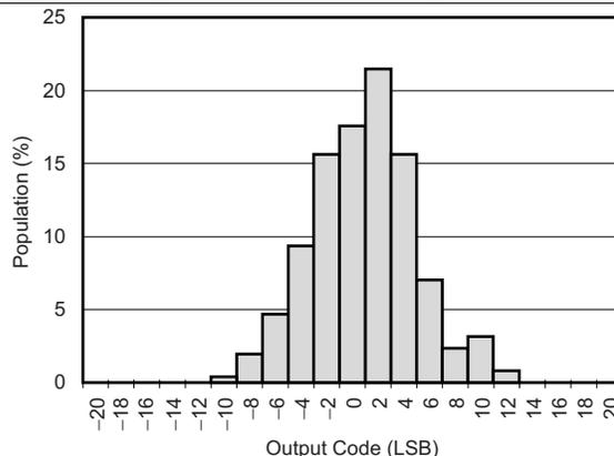
Gain = 64, data rate = 2.5 SPS, buffer = off, 256 readings
