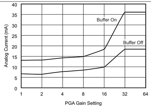
Figure 22. Analog Supply Current vs PGA Gain
