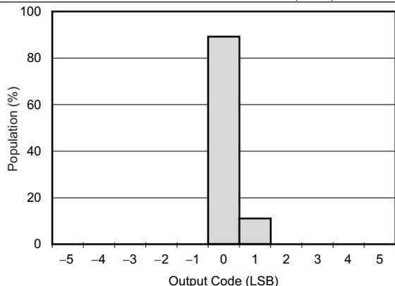
Gain = 1, data rate = 2.5 SPS, buffer = off, 256 readings
