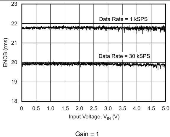
Figure 17. Effective Number of Bits vs Input Voltage
