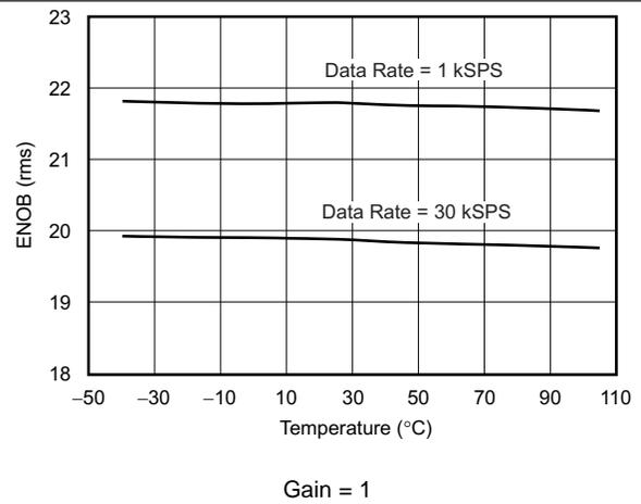
Figure 18. Effective Number of Bits vs Temperature
