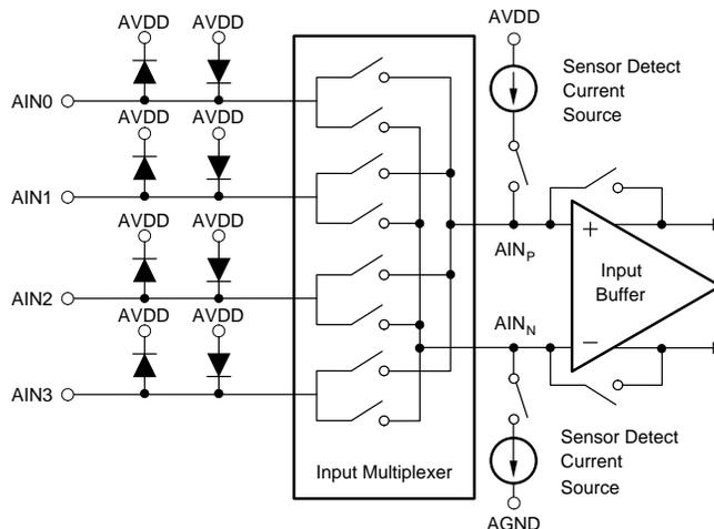
Figure 23. Simplified Diagram of the Input Multiplexer
