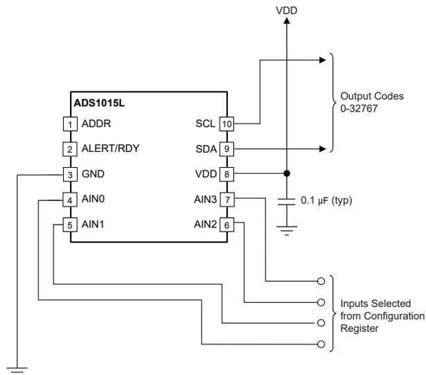
NOTE: Digital pin connections omitted for clarity.
