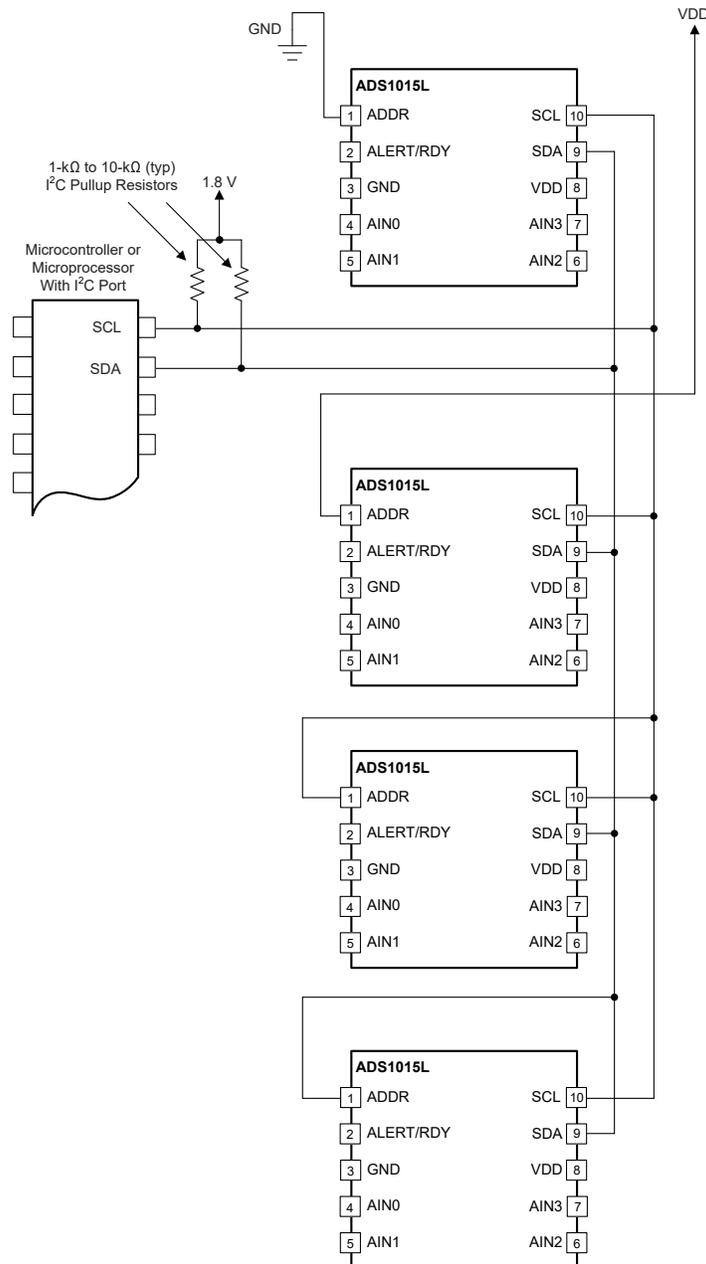
NOTE: The ADS101xL power and input connections are omitted for clarity. The ADDR pin selects the I<sup>2</sup>C address.
