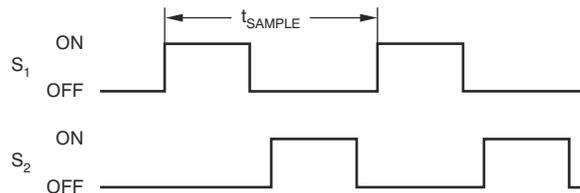
**Figure 7-5. S<sub>1</sub> and S<sub>2</sub> Switch Timing**
