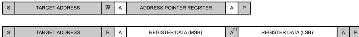
The controller can terminate the transmission after the first byte by not acknowledging.
