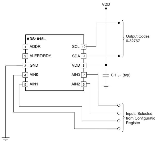
shows a single-ended connection scheme for the ADS1015L. The single-ended signal ranges from 0 V up to positive supply or +FS, whichever is lower. Negative voltages cannot be applied to these devices because the ADS101xL can only accept positive voltages with respect to ground. The ADS101xL do not lose linearity within the input range.
