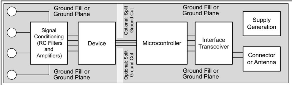
9-12 provides a good example of component placement, the best placement for each application is unique to the geometries, components, and PCB fabrication capabilities employed. That is, there is no single layout that is perfect for every design and careful consideration must always be used when designing with any analog component.
