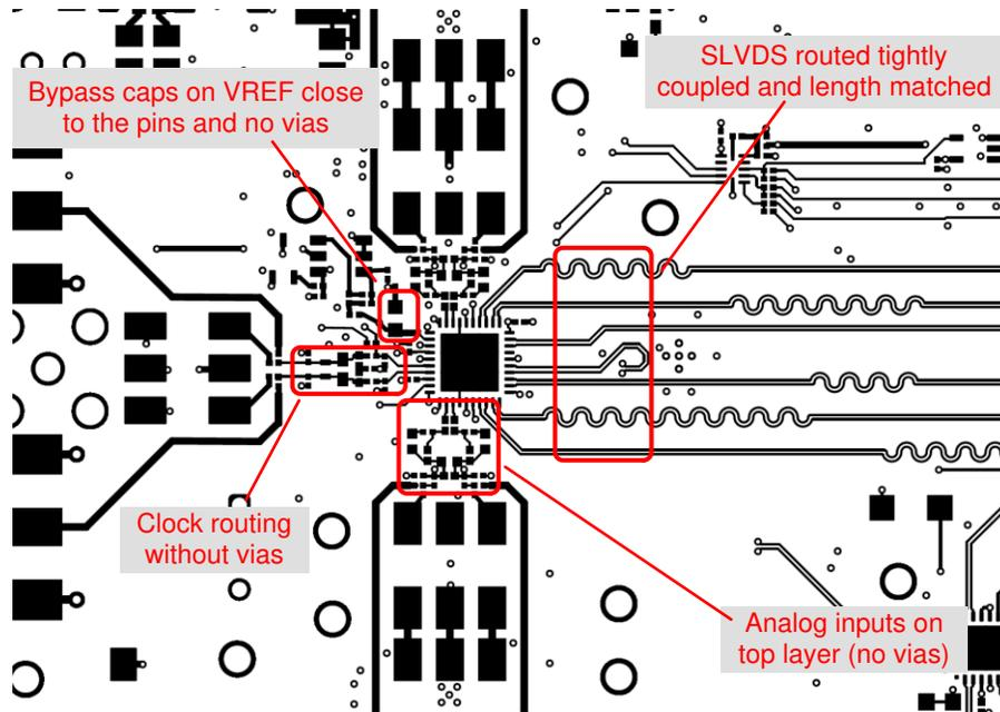
図 8-10. Layout example: top layer of ADC3683EVM
