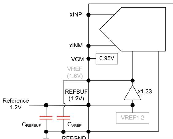
図 7-20. External 1.2V reference using internal reference buffer
