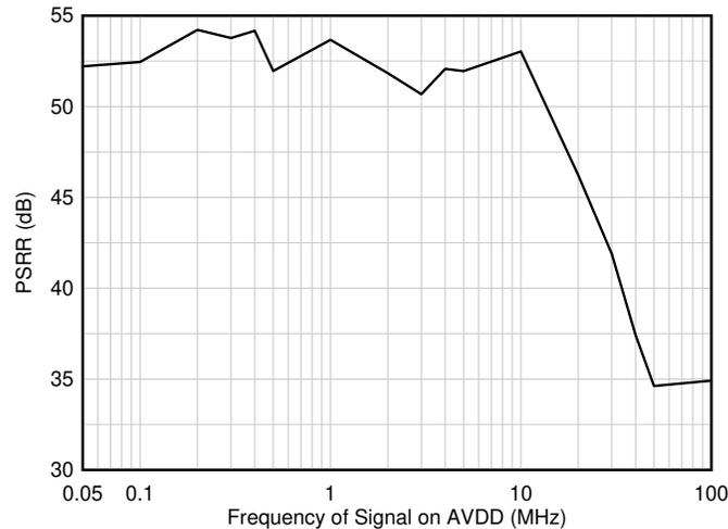
**図 8-7. Power supply rejection ratio (PSRR) vs frequency**
