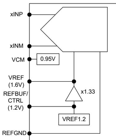
**Figure 7-17. Different voltage reference options for ADC3683-xEP**
