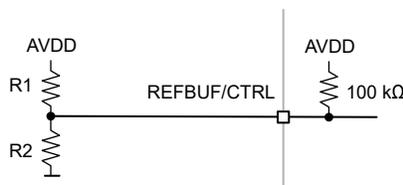
図 7-49. Configuration of external voltage on REFBUF/CTRL pin
