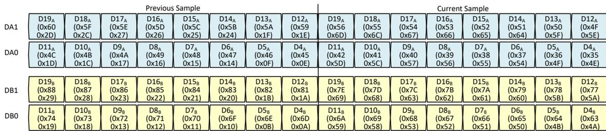
7-44. Example: 2-wire output bit mapping
