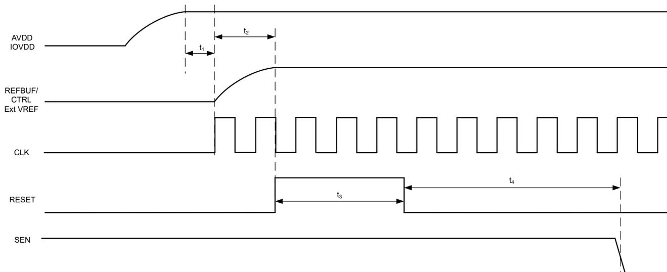
**図 8-6. Initialization of serial registers after power up**
