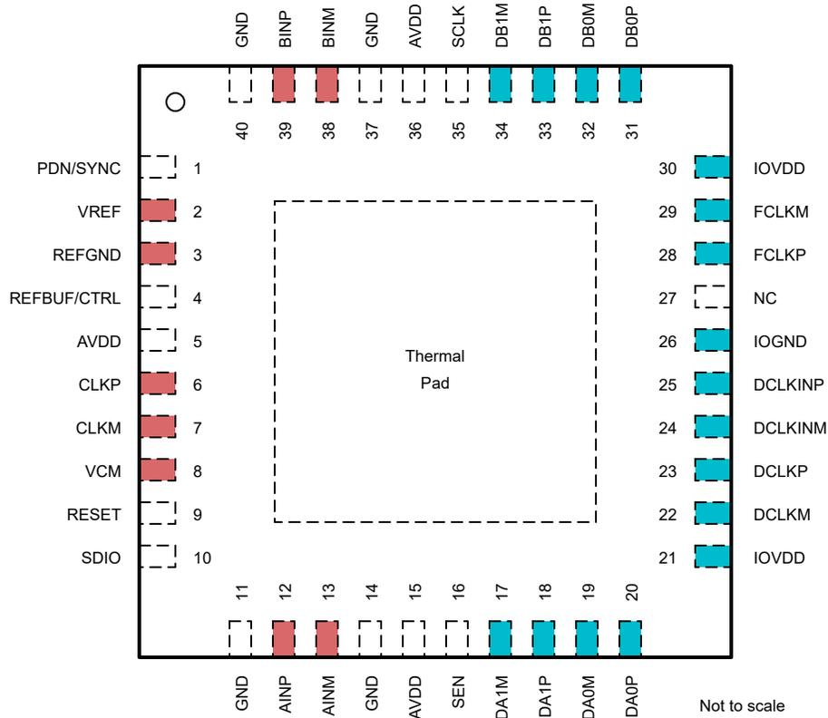
図 4-1. RSB (WQFN) Package, 40-Pin (Top View)
