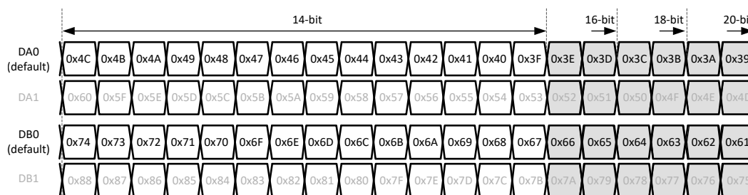
Figure 8-38. 1-wire output bit mapping
