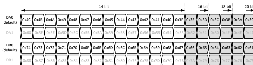
Figure 8-38. 1-wire output bit mapping
