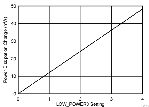
図 6-13. Power Dissipation Change vs LOW_POWER3 register setting
