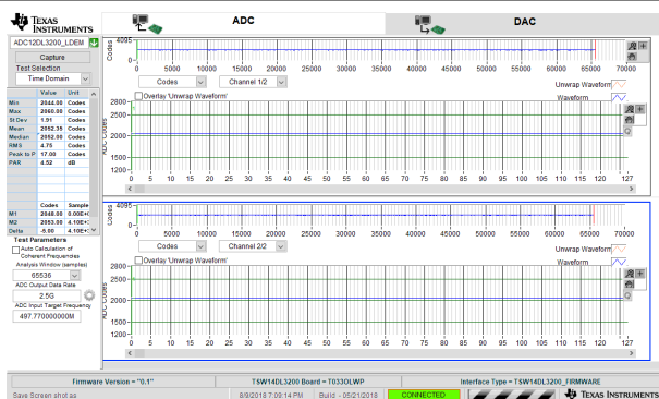
8-9. Idle-Channel Noise (No Input) for 2.5-GSPS, Dual-Channel Oscilloscope
