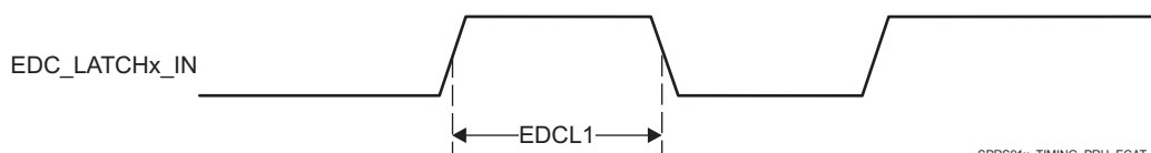
图 5-69. PRU-ICSS ECAT LATCHx_IN Timing
