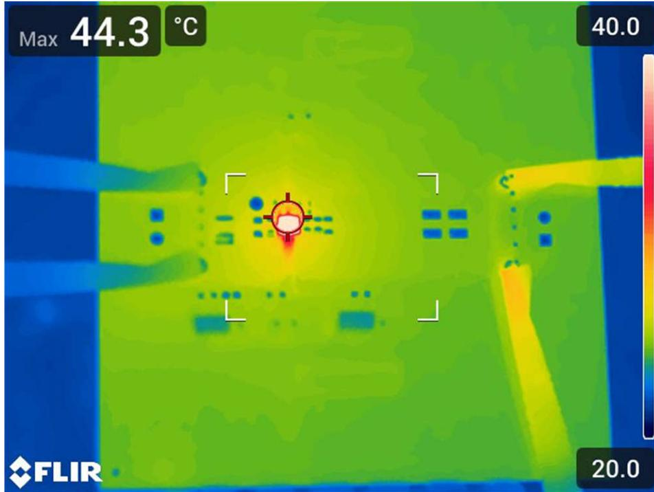
图 3-2. 热性能 ( TPSM82813PEVM-062 ,  $V_{IN} = 5V$  ,  $V_{OUT} = 1.8V$  ,  $I_{OUT} = 3A$  )
