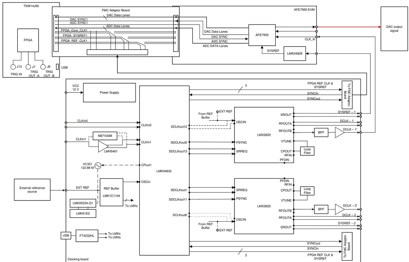
**图 2-8. Test Setup for AFE7950 Transmitter SFDR and IMD3 Measurement**
