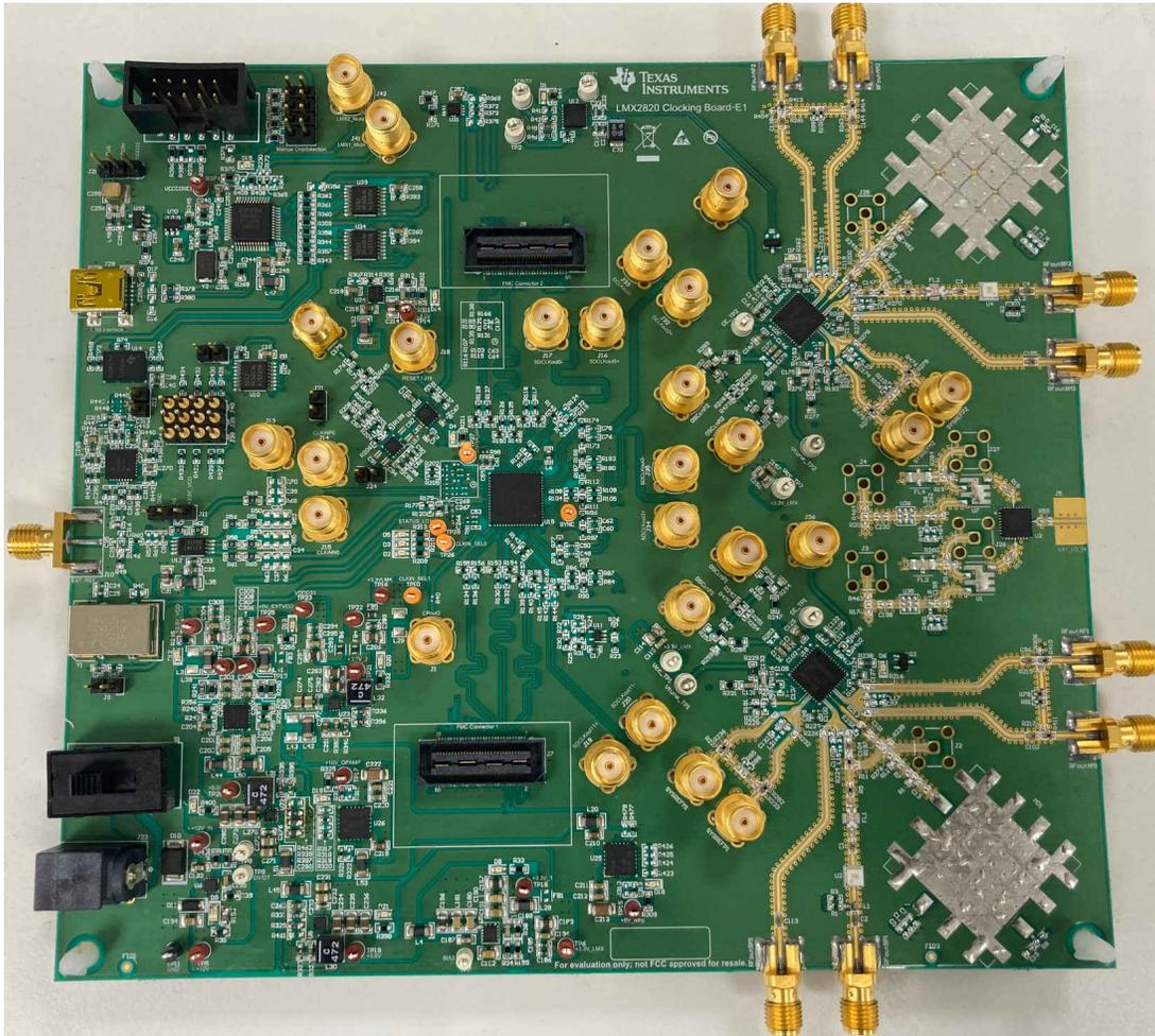
图 2-1. Multichannel Clocking Board
