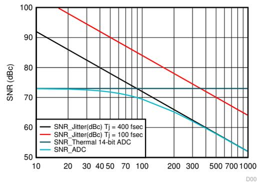
图 1-5. SNR Performance vs Input Frequency
