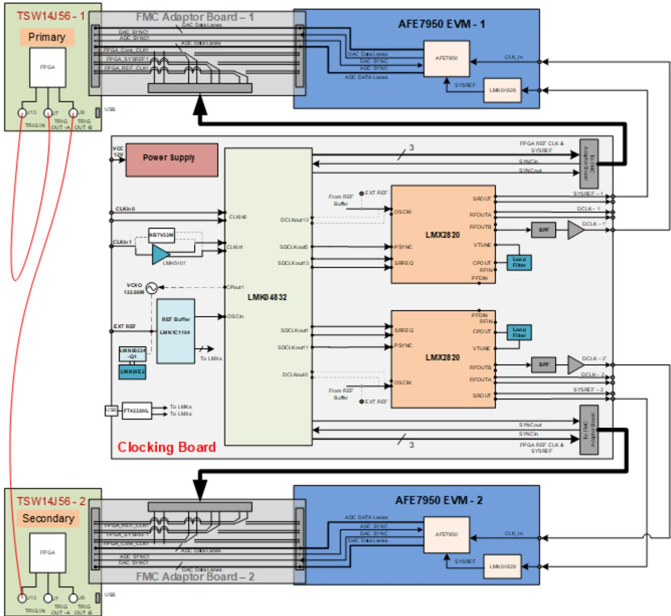
图 2-2. TIDA-010230 Device Synchronization Block Diagram
