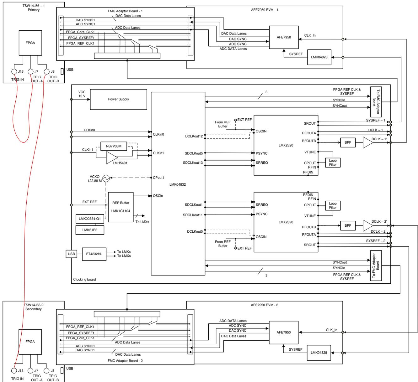
图 1-1. Block Diagram of Interface Between Clocking Board, AFE7950 EVM, FMC Adaptor Board, and TSW14J56 Board
