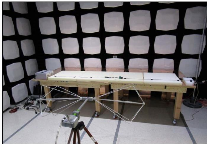
图 8 shows the test setup for conducted emissions with the LISNs (line impedance stabilization network) connections shown on the left side, they are the grey boxes.
