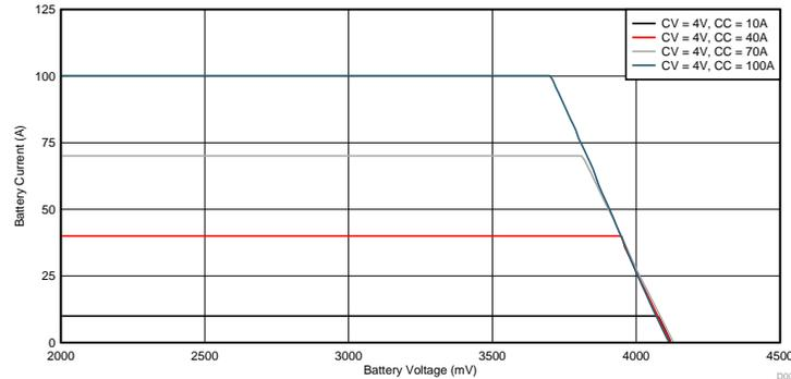
In 图 31, with the increase in current setting, the CC control will start transforming to CV control at lower voltage. The transformation remains linear throughout testing, indicating that the ability of the design to eliminate overcharging is not affected at higher currents.
