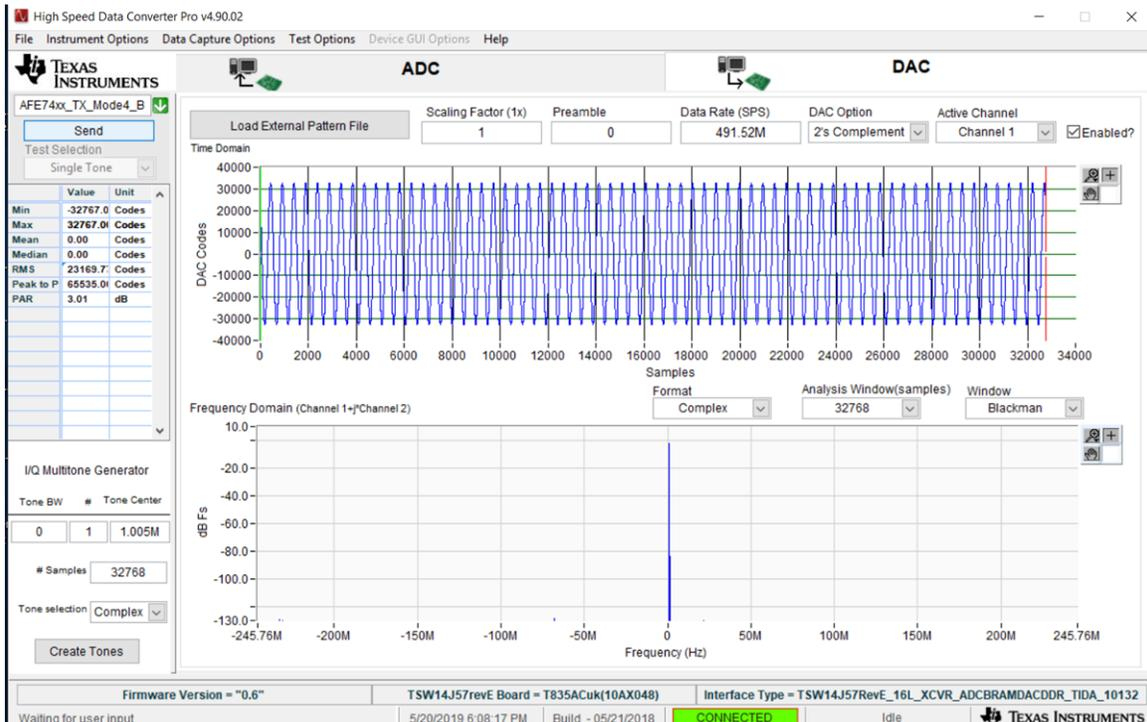
5. Load the *TIDA-010132\_AFE7444\_RX\_Mode9\_TX\_Mode4\_A\_B.cfg* file to configure the AFE7444 devices. Once the AFE7444 devices are programmed, D2 LED in the TSW14J57 card will begin blinking. If only the transmitter needs to be configured, skip step 6.
