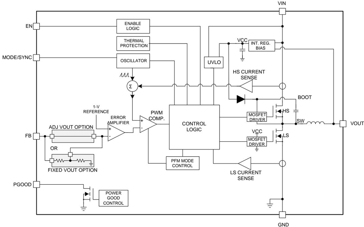
The LMZM23601 device is an integrated-inductor power module, that is specifically designed for space-constrained industrial applications. It is used in this design to bring down the 12-V input voltage to  $\pm 2.5$  V. It is available in two fixed output voltage options of 5-V and 3.3-V, and an adjustable (ADJ) output voltage option supporting a 2.5-V to 15-V range. The LMZM23601 has an input voltage range of 4-V to 36-V and can deliver up to 1000-mA of output current.
