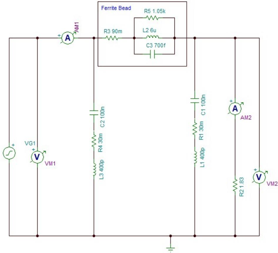
图 11. Insertion Loss of PI Filter
