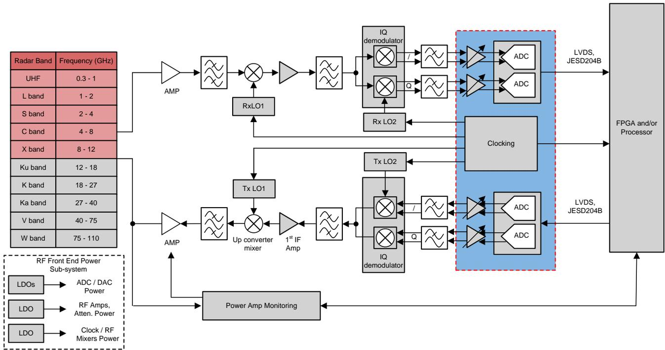
图 3. Wireless Communication Test Equipment AFE Subsystem
