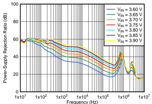
$I_{OUT} = 3\text{ A}$ ,  $C_{OUT} = 47\text{ }\mu\text{F} \parallel 10\text{ }\mu\text{F} \parallel 10\text{ }\mu\text{F}$ ,  $C_{NR/SS} = 10\text{ nF}$ ,  $C_{FF} = 10\text{ nF}$
