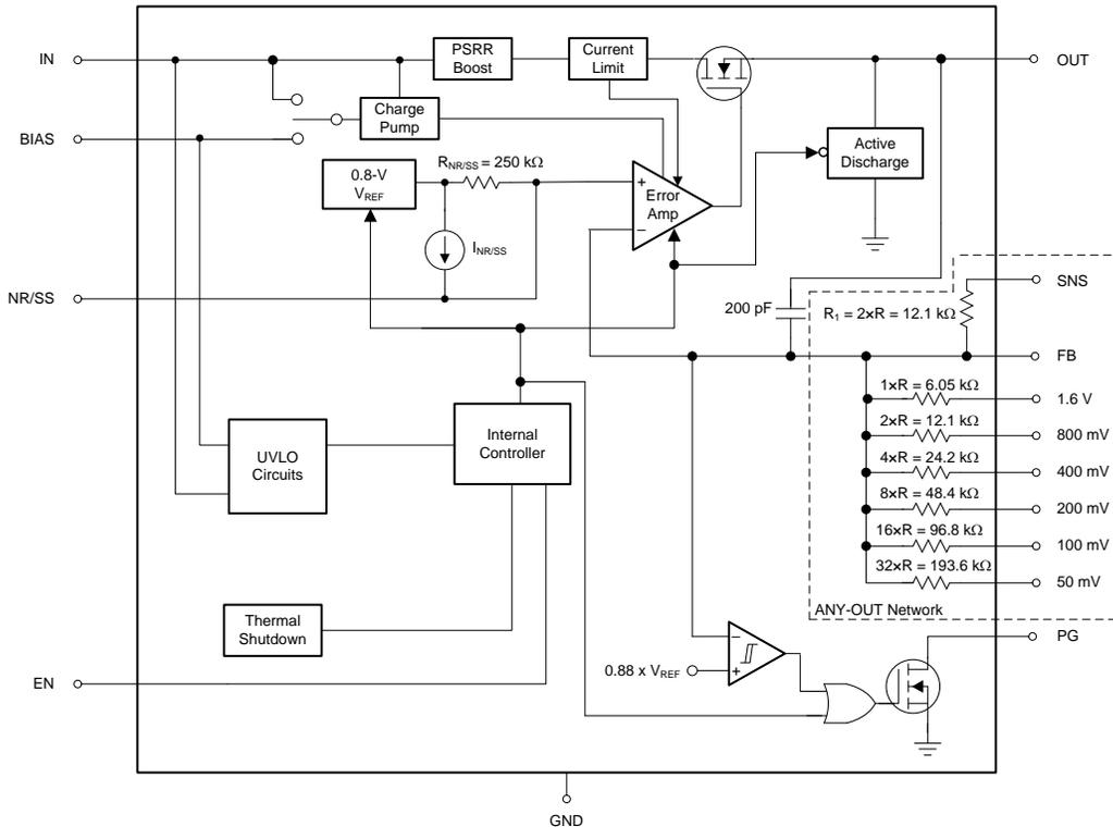
The TPS7A84 is a low-noise (4.4  $\mu V_{RMS}$ ), low-dropout linear regulator (LDO) capable of sourcing 3 A with only 180 mV of maximum dropout. The device output voltage is pin-programmable from 0.8 V to 3.95 V and adjustable from 0.8 V to 5.0 V using an external resistor divider.
