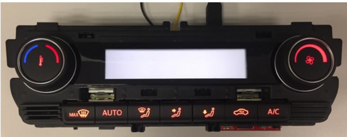
This TI design uses TPS7B4250-Q1 (tracking LDO) and SN74LV4051-Q1 (multiplexer, demultiplexer) to drive and multiplex the eight off board temperature (NTC) sensors.
