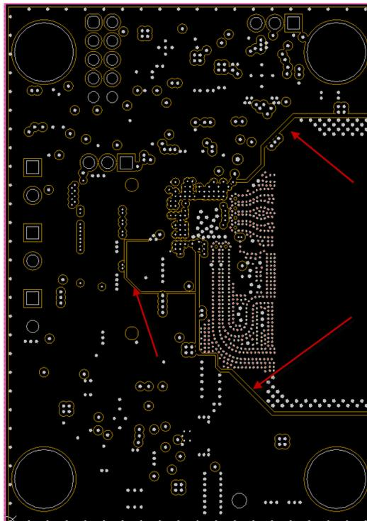
图 5. Cuts in Layer 2 Ground Plane
