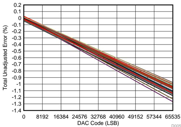
图 9. Total Unadjusted Error
