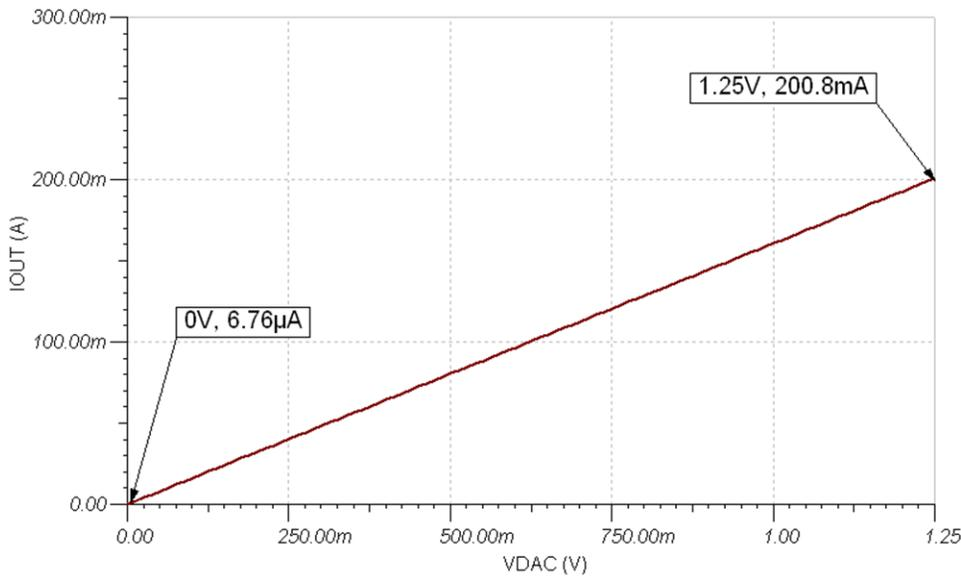
图 5. I<sub>OUT</sub> Transfer Function TINA-TI™ Simulation Software Results
