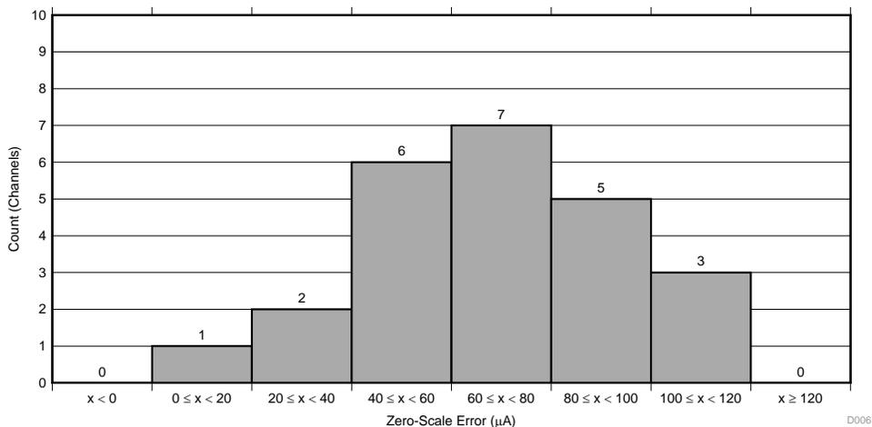
图 12. Zero-Scale Error Measurement
