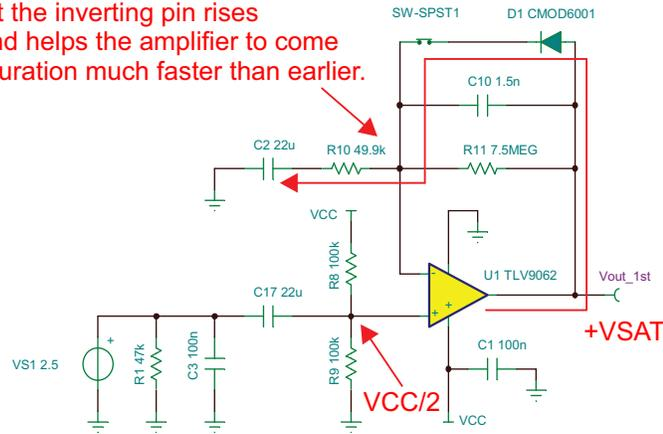
图 15. Power-on Settling Time Simulation With Diode
