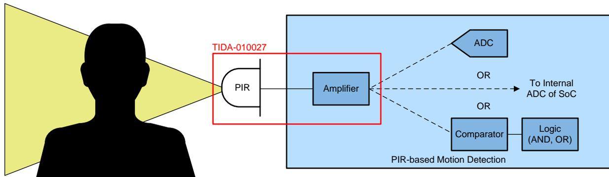
Any PIR-based motion detection circuit consists of several elements each with specific functions.
