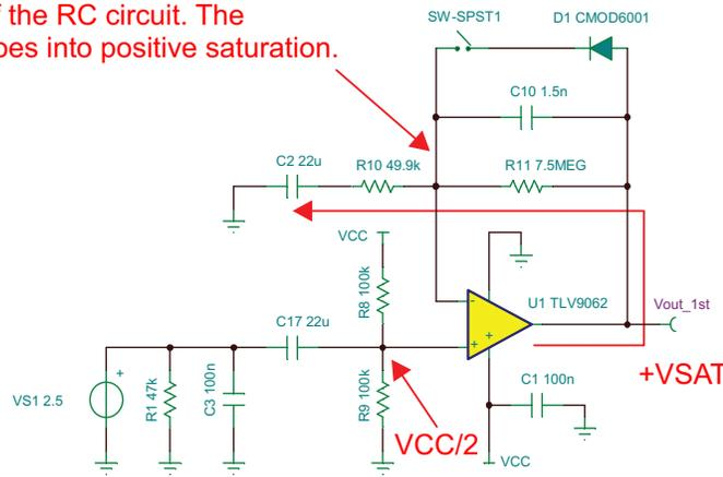
图 13. Power-on Settling Time Simulation Without Diode
