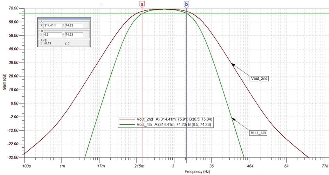
图 9. Frequency Response Dual vs Quad Stages (Linear Scale)
