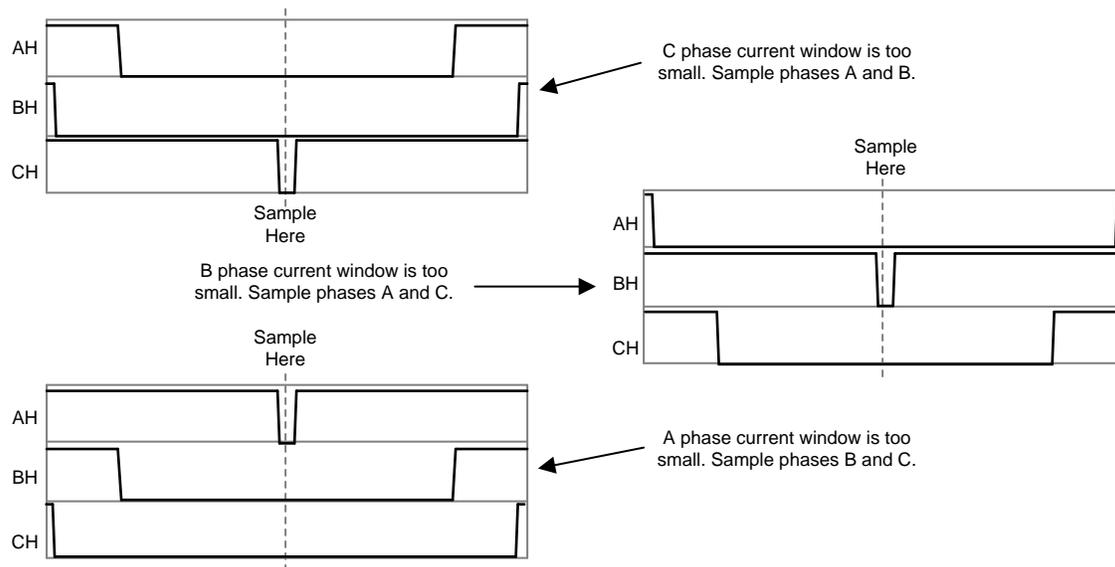
The two-shunt current measurement technique uses the principle of Kirchhoff's current law (KCL), which is that the sum of the currents into a single node equals zero. By measuring only two-phase currents, the third is calculated with KCL. 图 3 shows a circuit for the two-shunt current measurement technique.
