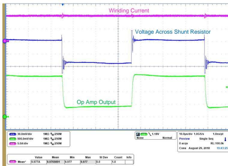
图 28. Step Response of Current-Sensing Circuit With 10-A Positive Current
