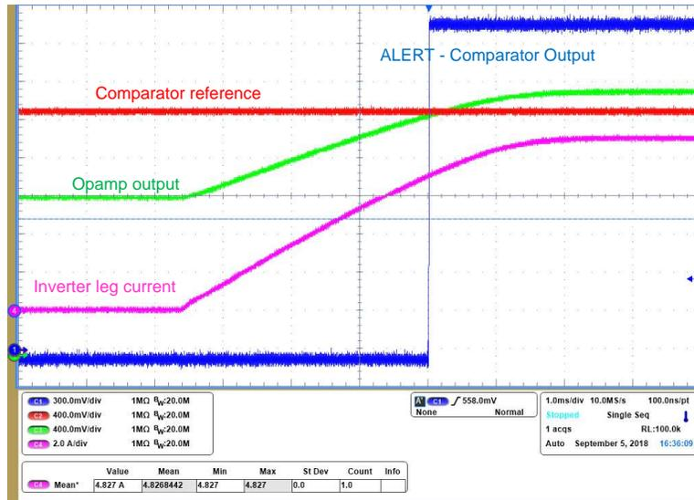
图 44. Overcurrent Detection for Positive Current at 2.0  $\mu$ s/div
