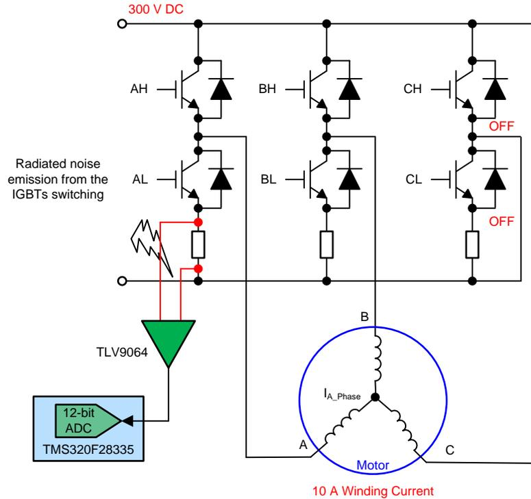
The DC bus voltage is set at 300 V, and the winding current is at 10 A. PWM is applied to Phase A and Phase B. Phase C is left open. 图 37 shows the PWM signals, the PWM signal driving the high-side IGBT for Phase A has 10% duty, and the low-side IGBT is kept off. The PWM signal driving high-side IGBT for Phase B has 2.5% duty, and the frequency is set at 15 kHz.
