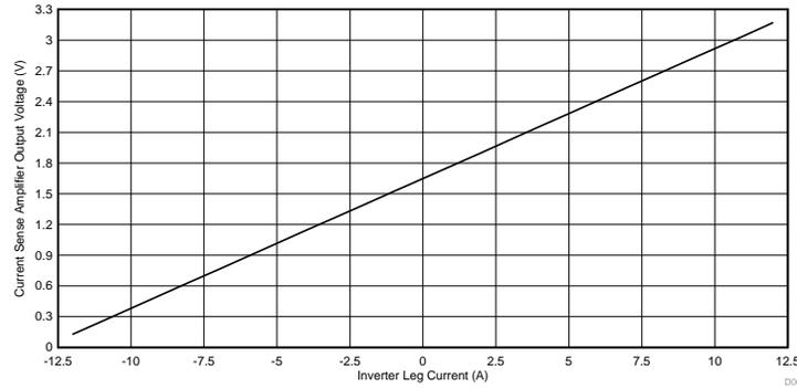
With the purpose of evaluating the transfer function for actual data used in the sensorless FOC algorithm, 图 33 shows the transfer function of the inverter leg current through the shunt resistor versus the values read from ADC data buffer of TMS320F28027F. The transfer function is linear across -12 A to +12 A current. The transfer function is also linear, which means no extra calibration algorithm needed.
