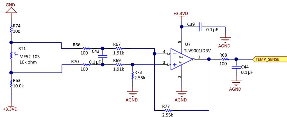
The ADC of the MCU reads the output of the temperature sense signal-conditioning circuit and necessary action can be taken for overtemperature protection.
