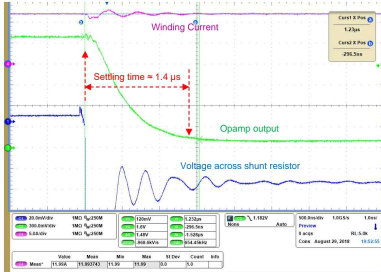
图 31. Step Response of Current-Sensing Circuit With 12-A Negative Current
