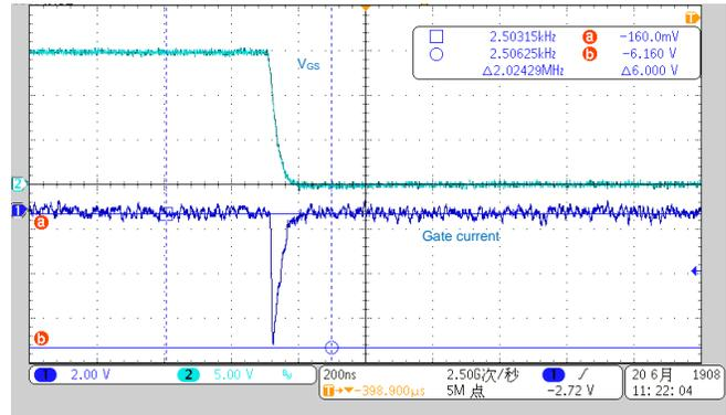
图 23. Source and Sink Current From Gate Driver
