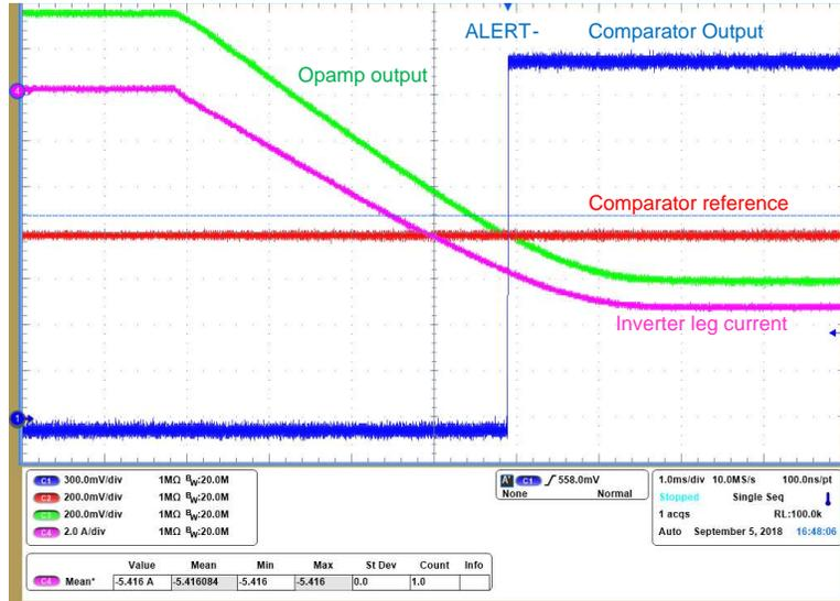
图 46. Overcurrent Detection for Negative Current at 2.0 ms/div
