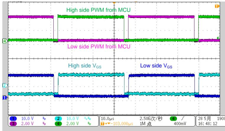
图 20 shows the PWM signals of high-side and low-side gate to source voltage from UCC27712, which shows that the dead time configured by the MCU at both of the edges of the PWM. The dead time is programmed to 2  $\mu$ s.
