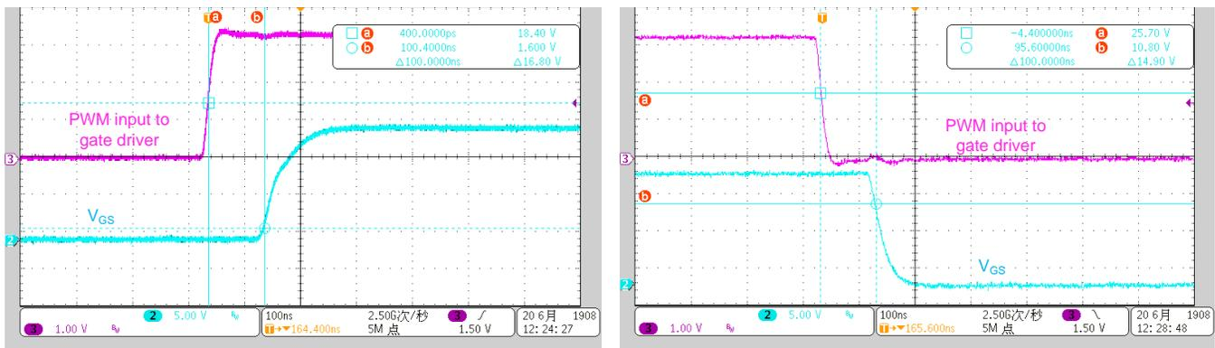
图 25 shows the UVLO protection of UCC27712, and the threshold voltage observed is approximately 8.4 V, which ensure that the IGBT is turned on properly with sufficient gate voltage.
