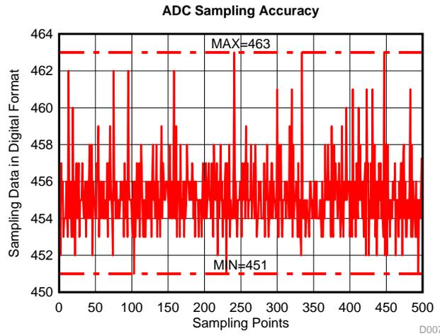
图 41. ADC Sampling Points Distribution
