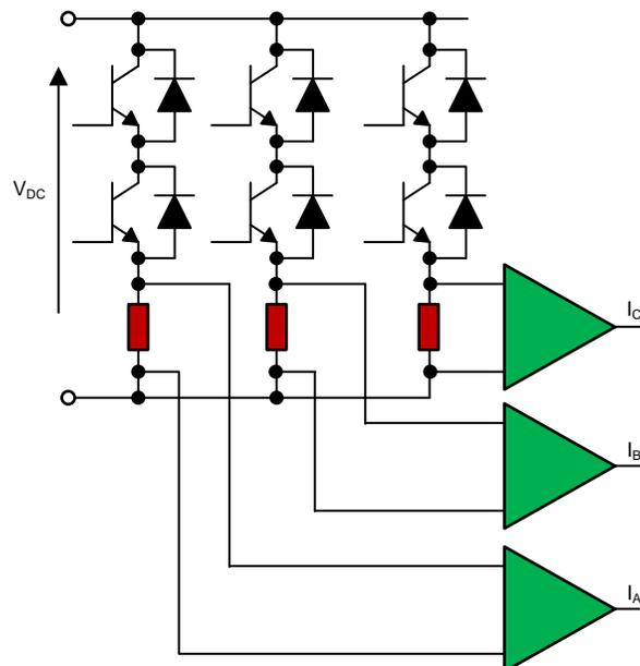
图 2. Using Three-Shunt Current Sampling Technique
