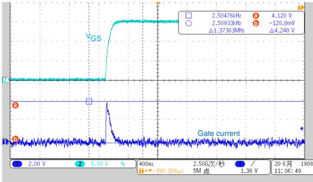
图 22. Sink Current From Gate Driver
