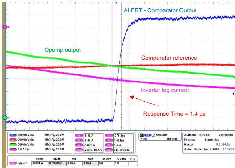
图 47 shows the overcurrent protection in hardware, which is achieved by pulling up the active-low enable pin of line driver SN74AHC367. 图 48 shows the response time from overcurrent detection comparator output to the IGBT gate turn off.
