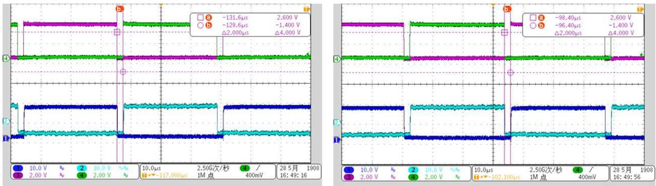
图 21, 图 22, and 图 23 show the source and sink current provided by UCC27712. The peak gate current is captured by monitoring the voltage across the gate resistors. The test conditions follow:
