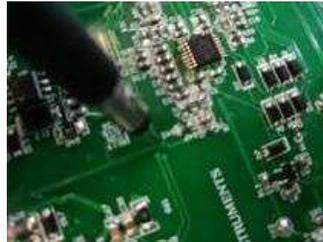
图 39 shows the test results of noise effect on current sense amplifier, the floating probe near amplifier input shows DC shift and noise oscillation due to IGBTs switching. Noise is also observed on the amplifier output.
