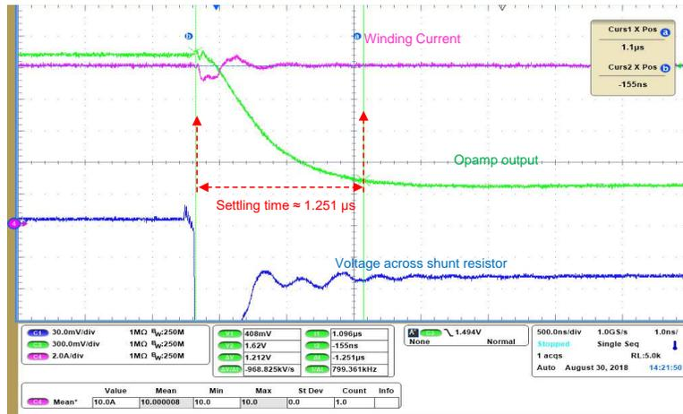
图 29. Step Response of Current-Sensing Circuit With 10-A Negative Current
