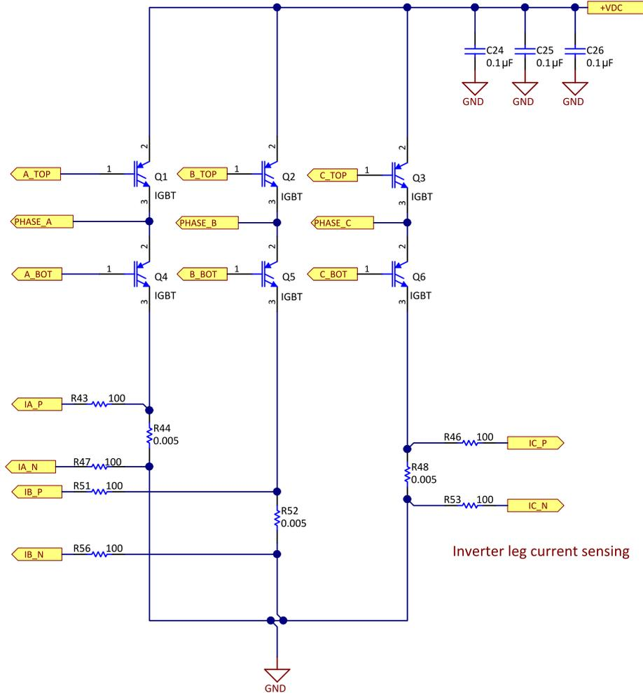
图 8. DC Bus Capacitor Placed in Reference Design Board
