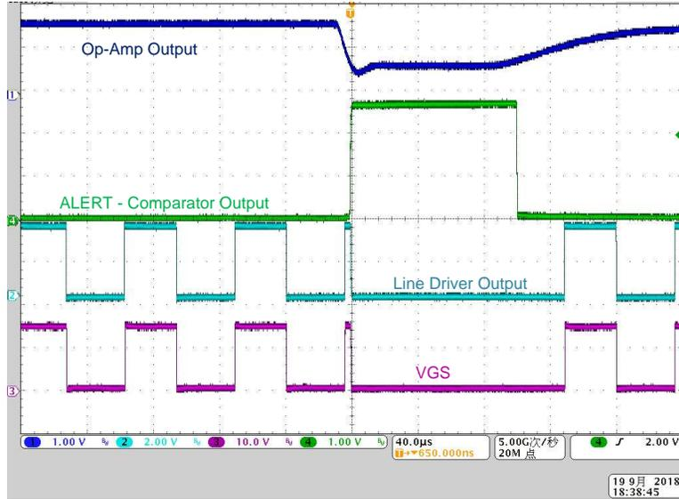
图 48. Response Time of Overcurrent Protection in Hardware
