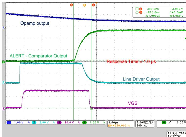
The response time of the overcurrent detection is less than 1.0 μs in hardware protection, which is fast enough to protect an IGBT (IGBTs typically have more than a 5-μs short-circuit capability). The lowest propagation delay of gate driver and line driver enables the fast turnoff of the IGBTs during an overcurrent event.
