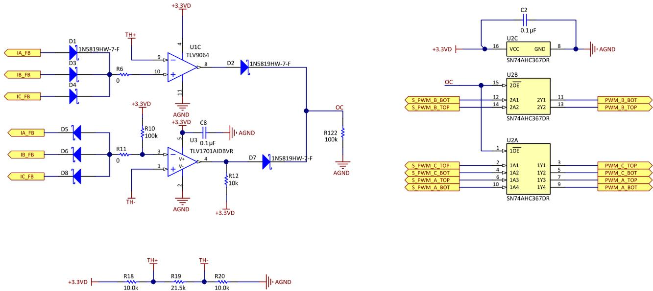
The overcurrent protection circuit output signal OC is connected to the enable pin of the line driver device - SN74AHC367. Once the overcurrent event occurs, the OC signal will be pulled up and disable the output of the line driver and hence the SVPWM signals at the input of gate driver - UCC27712. Thus, the process of protection is achieved all by hardware, which features very fast response time.
