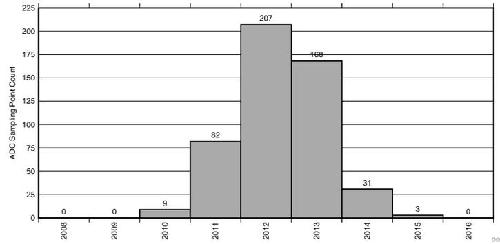
The error variation when using a LDO as the power supply is 4 codes, which means the error of the output of the amplifier is effected by the ripple in the ADC reference which is divided from 3.3-V power supply. If the designer need more accurate ADC data, it is recommended to use a LC filter at the ADC reference voltage input.
