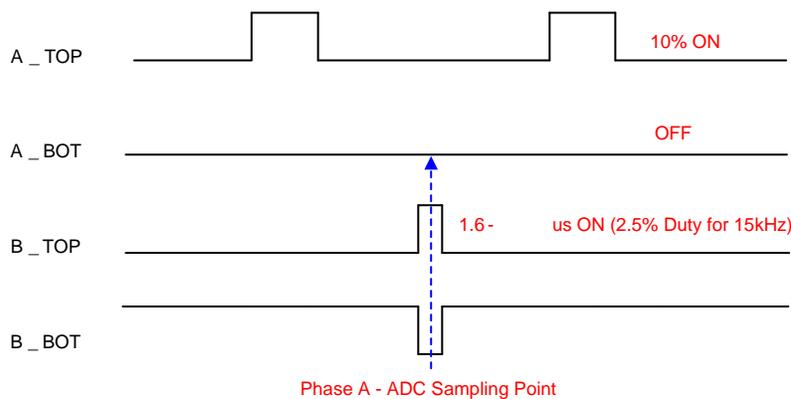
During the testing the ADC of the MCU samples the current sense amplifier output at the middle of phase A high side off period, which is falling near the IGBT switching of phase B, meaning the noise generated during the IGBT switching will couple to the current sense amplifier circuit. The radiated noise emission signal is captured by a floating probe close to the input path of the current sense amplifier, which 图 38 shows.
