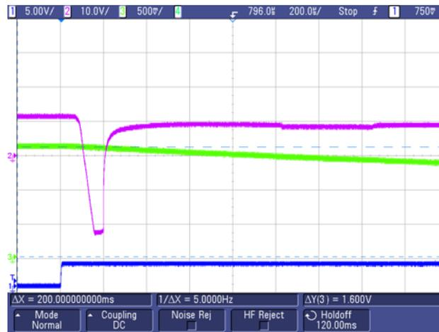
A detail of the motor voltage transition on lumbar pump turn off shows the amplitude and duration of the inductive *kick* caused by turning off the motor. The duration of the negative pulse is about 100 microseconds. The negative pulse is clamped at about 23 V. Zener diode D5 has a nominal breakdown point of 21 V; the remainder of the voltage drop is due to the blocking diode D6.
