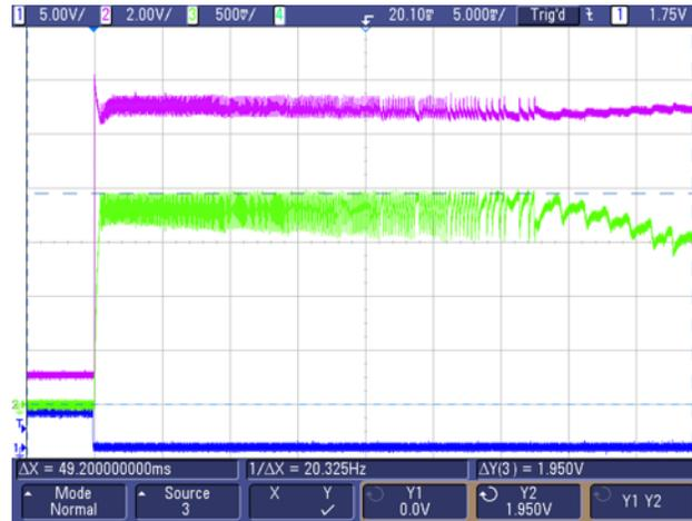
The DRV8873-Q1 current limit threshold is set to 6.5 A  $\pm$ 1 A when ITRIP\_LVL is set to 10b. The value of 330  $\Omega$  for R14 (in this case) and scale factor of 1125 A/A on the IPROP signal gives a scale factor of 3.4 A of motor current per volt of signal on ISense8873. The measured maximum value of 1.95 V of ISENSE (after the MUX) indicates the current is limiting at a value of:
