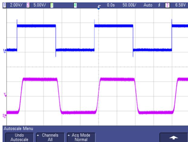
At this scale, there is no observable time delay between transitions on the TXD pin and transitions on the LIN pin. The controlled slope of the LIN bus signals is also apparent. For this measurement, a 1-kΩ resistor to VBATT was applied to the LIN bus line, as would normally occur when connected to a master node. See also
