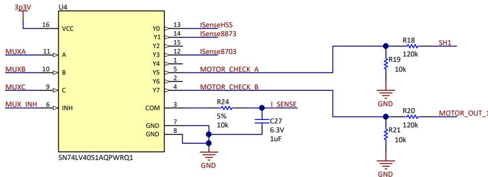
In this design, only five of the eight channels are used; in a full power seat design, additional channels would be used to monitor the signals associated with additional motor drives. By setting the MUXA, MUXB, and MUXC signals, the microcontroller ADC can monitor:
