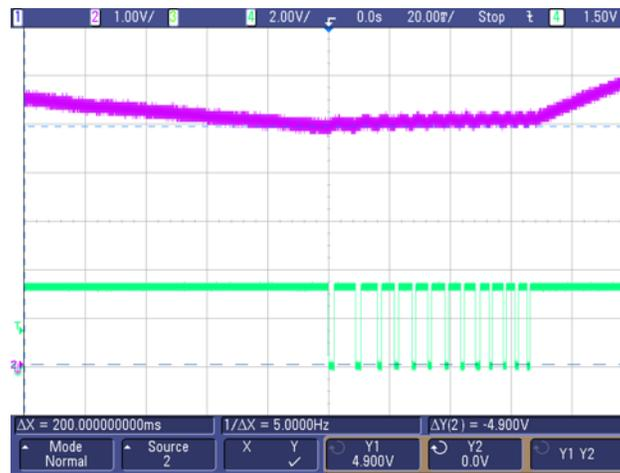
Channel 4 shows the reaction of the OK\_8873 signal to the drooping VBATT. When the motor current first droops to about 4.9 V, the DRV8873-Q1 FAULT open-drain output signal activates, pulling the OK\_8873 signal to a logic low level.
