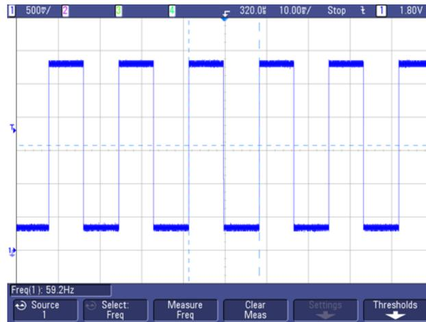
The frequency of the Hall effect sensor signal is used to measure the motor speed for various levels of applied supply voltage VBATT. 图 23 shows the results of this testing. As expected, the speed increases as the applied VBATT voltage level increases. The relationship is relatively linear across the expected range of operation, with some variation due to mechanical factors such as the friction of the gears.
