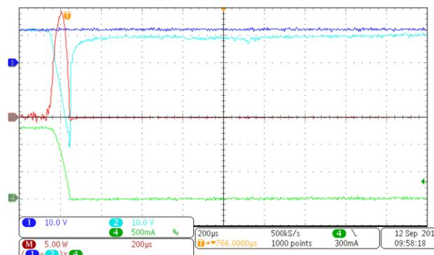
The TPS2H160-Q1 specifies an absolute maximum of 40 mJ for "Inductive load switch-off energy dissipation, single pulse, single channel", so this energy that must be dissipated each time the lumbar pump motor is turned off is significantly less than the specified value. Designers can use the TPS2H160-Q1 for this application without the need for protection diodes D5 and D6, unless the motor is significantly larger than the model used for testing.
