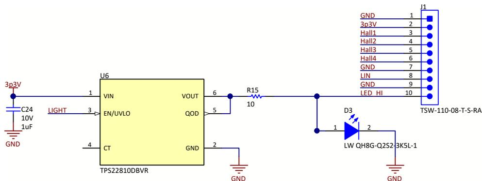
The LED D3 is selected to have a relatively low turn-on voltage, allowing current-limiting resistor R15 to be used in series with the LED.
