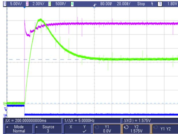
Channel 1 shows the signal on SWITCH1 going low when the button is pushed. Channel 2 shows the motor voltage; Channel 3 shows the ISense\_HSS signal which corresponds to the current through the high-side switch to the pump motor.
