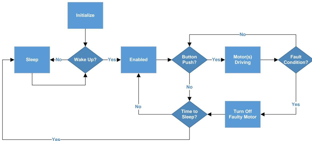
When a button is pushed, the microcontroller sets the corresponding GPIO pins to control the actuator associated with the desired action. At this point the analog multiplexer (MUX) is also set to connect the active drive circuit to the ADC of the microcontroller. In testing mode, the actuator is active as long as the button is pushed, unless a fault condition occurs.
