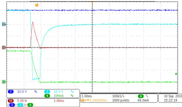
The TPS2H160-Q1 specifies an absolute maximum of 40 mJ for "Inductive load switch-off energy dissipation, single pulse, single channel", so this energy that must be dissipated each time the solenoid valve is turned off is significantly less than the specified value. Designers can therefore use the TPS2H160-Q1 for this application without the need for external protection diodes.
