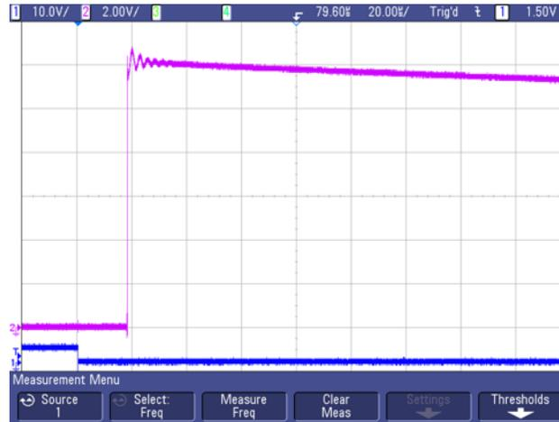
Channel 1 is the pushbutton signal, channel 2 is the voltage applied to the motor. The delay between button push and application of motor voltage is about 20 ms. The motor voltage increases rapidly to about 12 V, with a small ringing on the rising edge. The motor voltage of approximately 12 V indicates there is not a significant voltage drop across the active full-bridge MOSFETs, due to the low  $R_{DS(ON)}$  of the MOSFETs selected.
