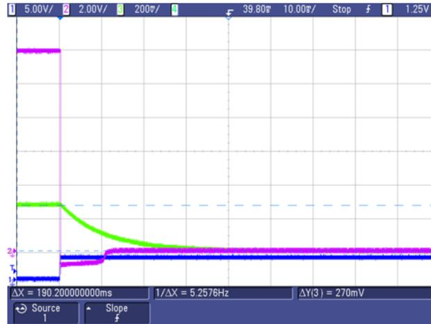
图 35 shows an expanded view of the signal waveforms during lumbar valve solenoid turn off. The solenoid voltage on Channel 2 transitions to a negative value due to the inductive energy stored in the solenoid windings. The negative voltage level is clamped to about  $-0.7\text{ V}$  by the external diode supplied with the lumbar valve.
