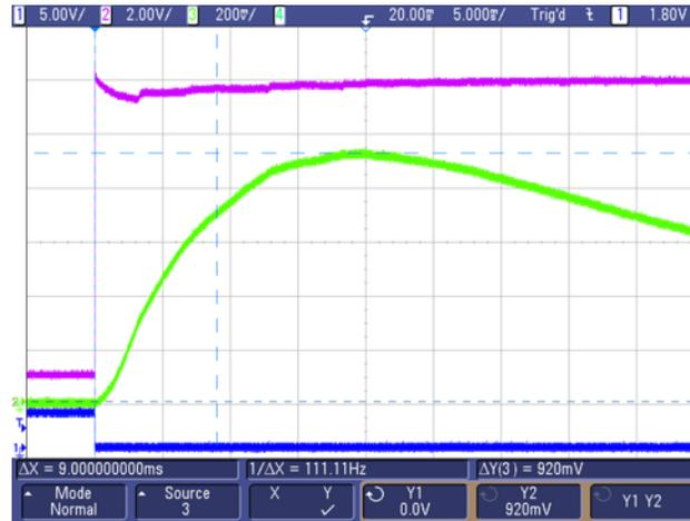
As the motor accelerates, the back EMF produced by the motor increases, reducing the current through the motor. This is seen in the current trace (Channel 3) when the ISENSE signal amplitude reduces below the maximum value.
