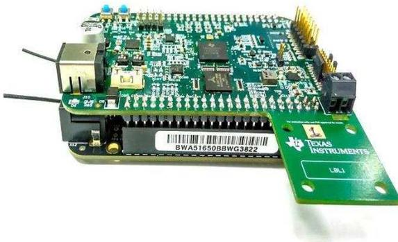
图 26. DSP Board Sitting on top of BeagleBone™ Black Wireless With DC Jacks Aligned
