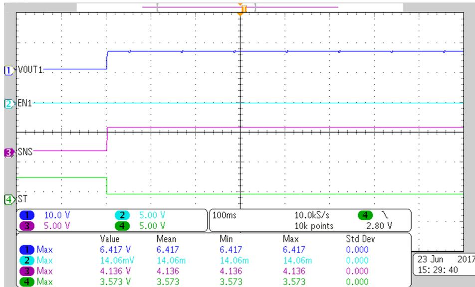
图 5. Open-Load With Switch-Disabled Test Results
