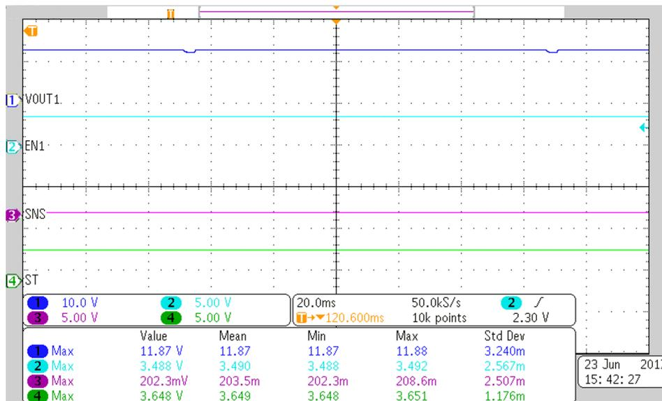
图 4. Open-Load With Switch-Enabled Test Results
