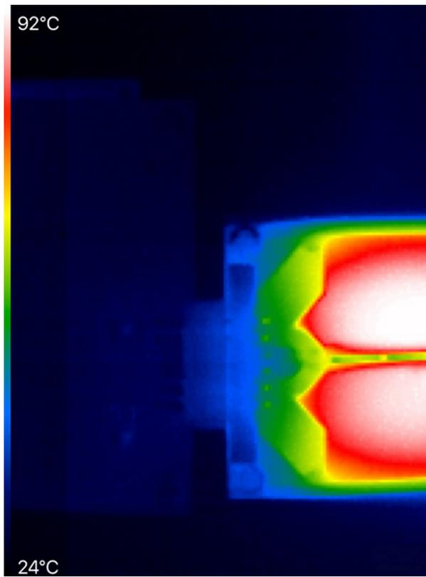
图 7. TPS1HA08-Q1 Thermal Performance Test Results
