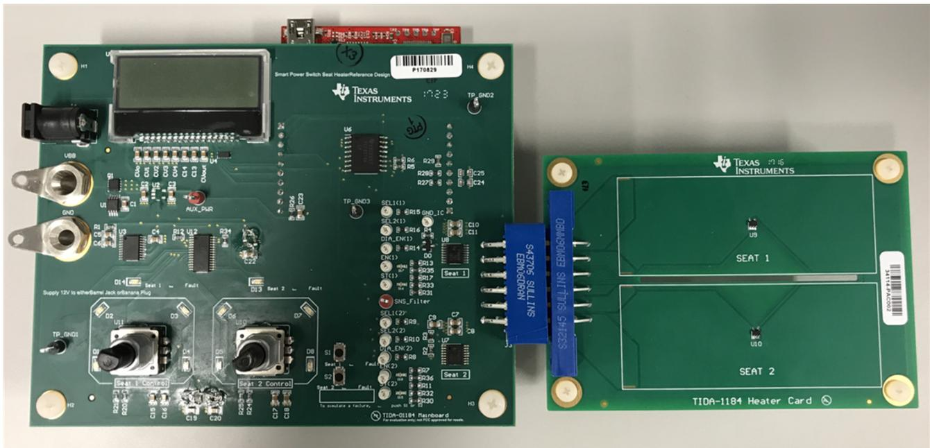
图 2. Default Board Setup With Heater Card Attached
