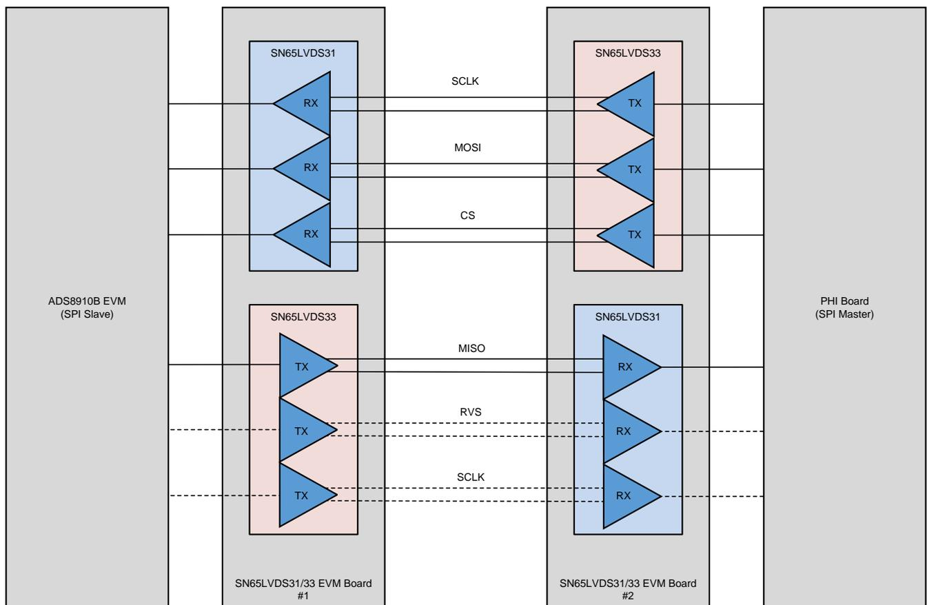
图 7. Eliminating Round-Trip Delay Block Diagram
