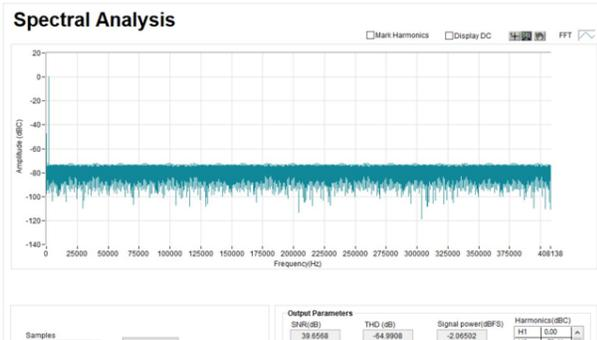
图 15. Single-ended Spectral Analysis Sample
