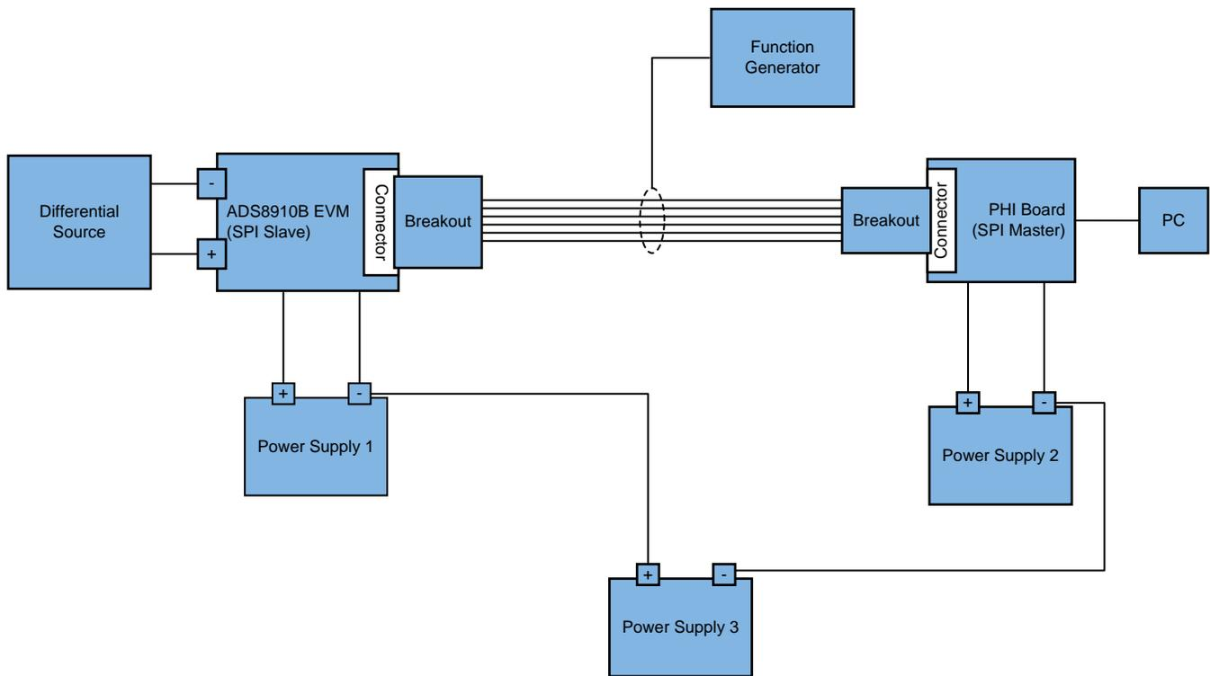
图 12. Single-ended SPI Test Setup
