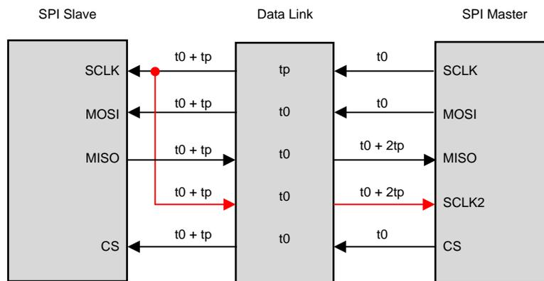
图 8. Feed SCLK back to SPI Master
