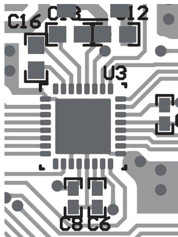
图 39. Bypass Capacitors of AVDD and DVDD
