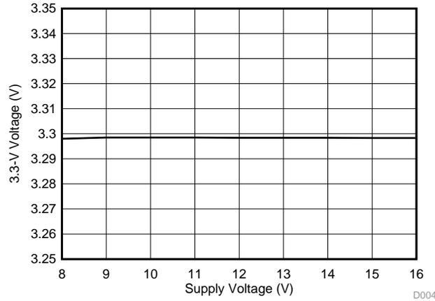
图 14. 3.3-V Voltage With Supply Voltage
