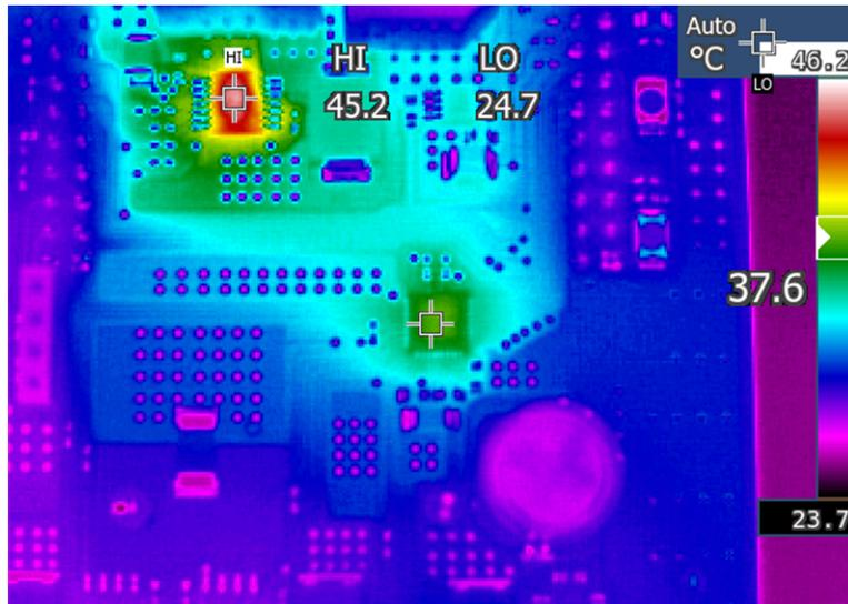
图 32. Motor and Clutch Thermal Test
