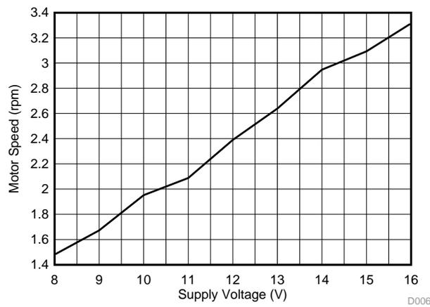
图 30. Motor Speed With Supply Voltage
