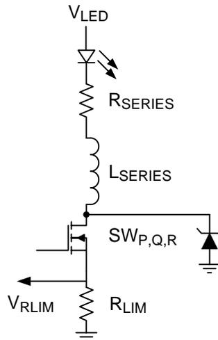
图 7. Parasitic Inductance ( $L_{series}$ ) and Resistance ( $R_{series}$ ) in Series With LED
