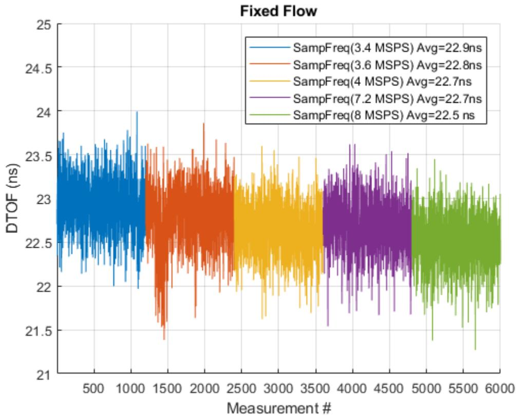
图 25. DToF of 1 GPM at Different Sampling Rates
