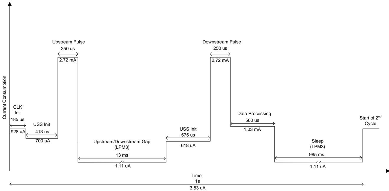
图 26. Profile of Current Consumption During Duration of Measurement
