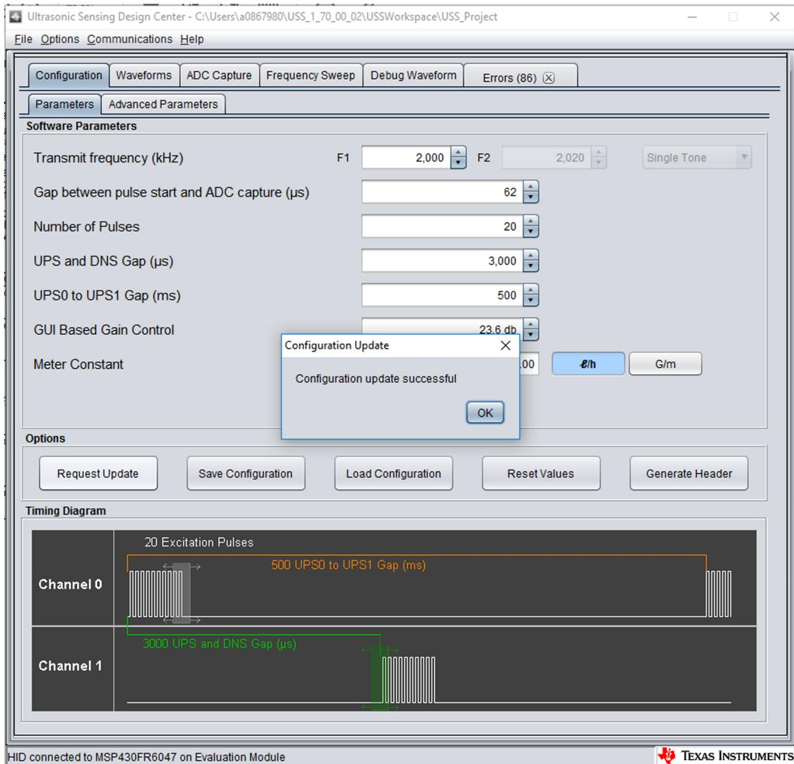
图 18. Loading Configuration to Device From GUI
