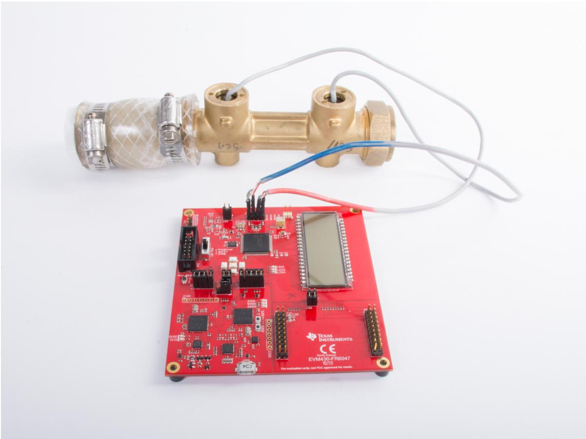
图 14. EVM430-FR6047 Connected to Water-Flow Meter in Stationary Setup
