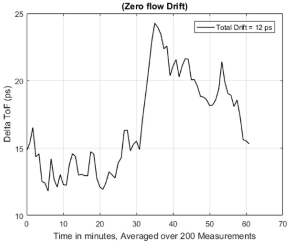
图 23. Zero Flow Drift of DToF With EVM430-FR6047 In-Oven
