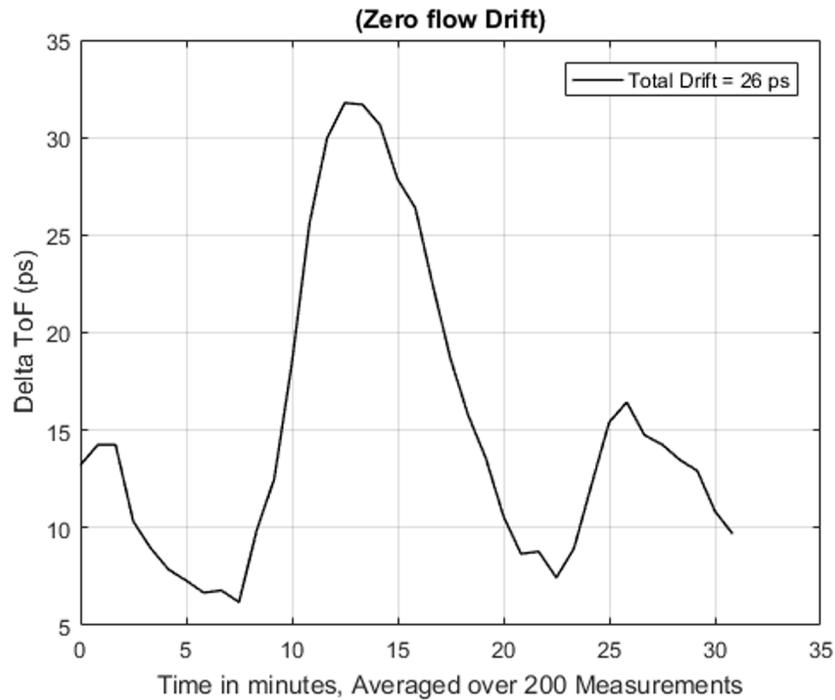
图 22. Zero Flow Drift of DToF With Meter In-Oven
