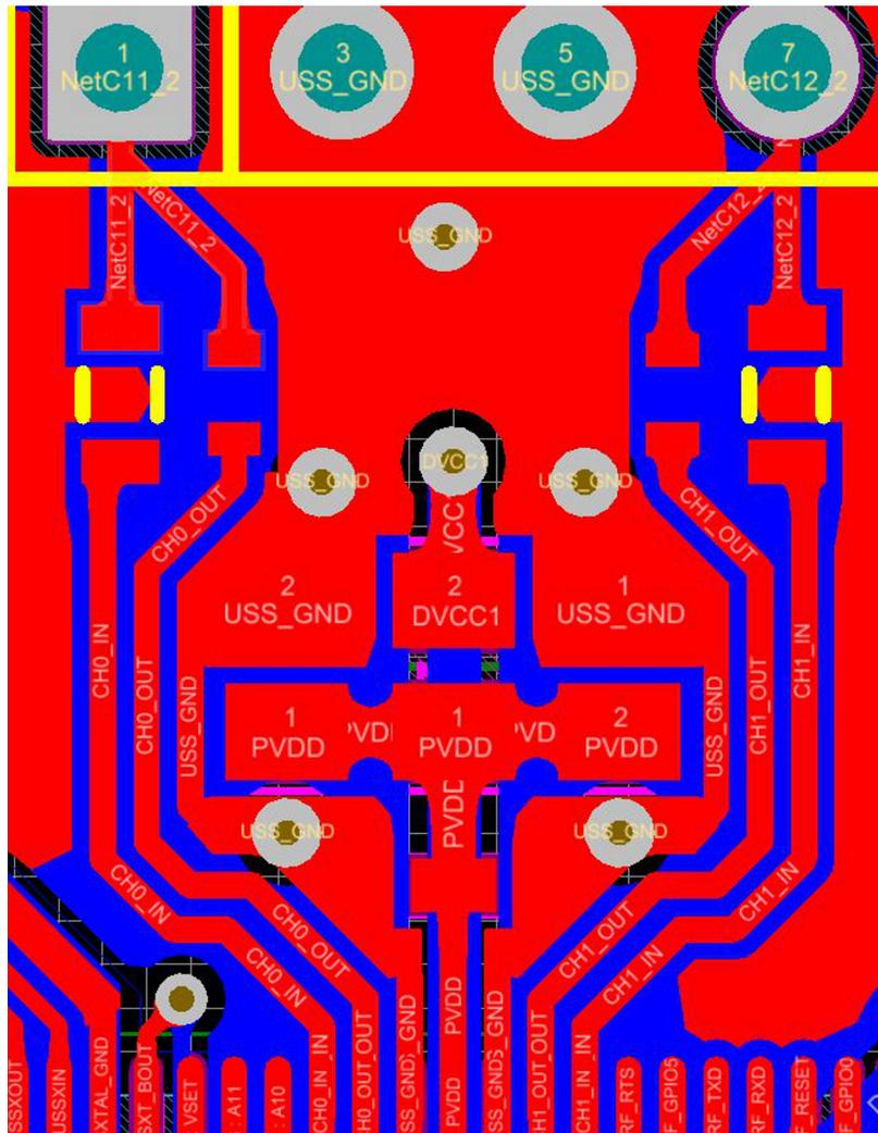
图 28. Layout Guidelines: Transducer Symmetric Traces
