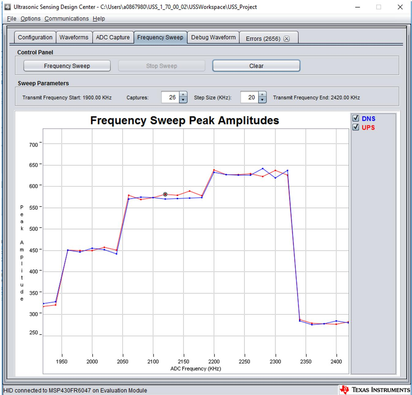
图 15. Frequency Response Test Results
