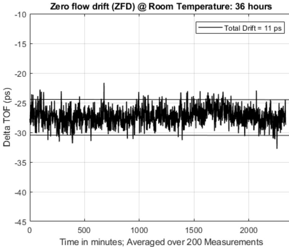
图 21. Zero-Flow Drift of DToF at Room Temperature
