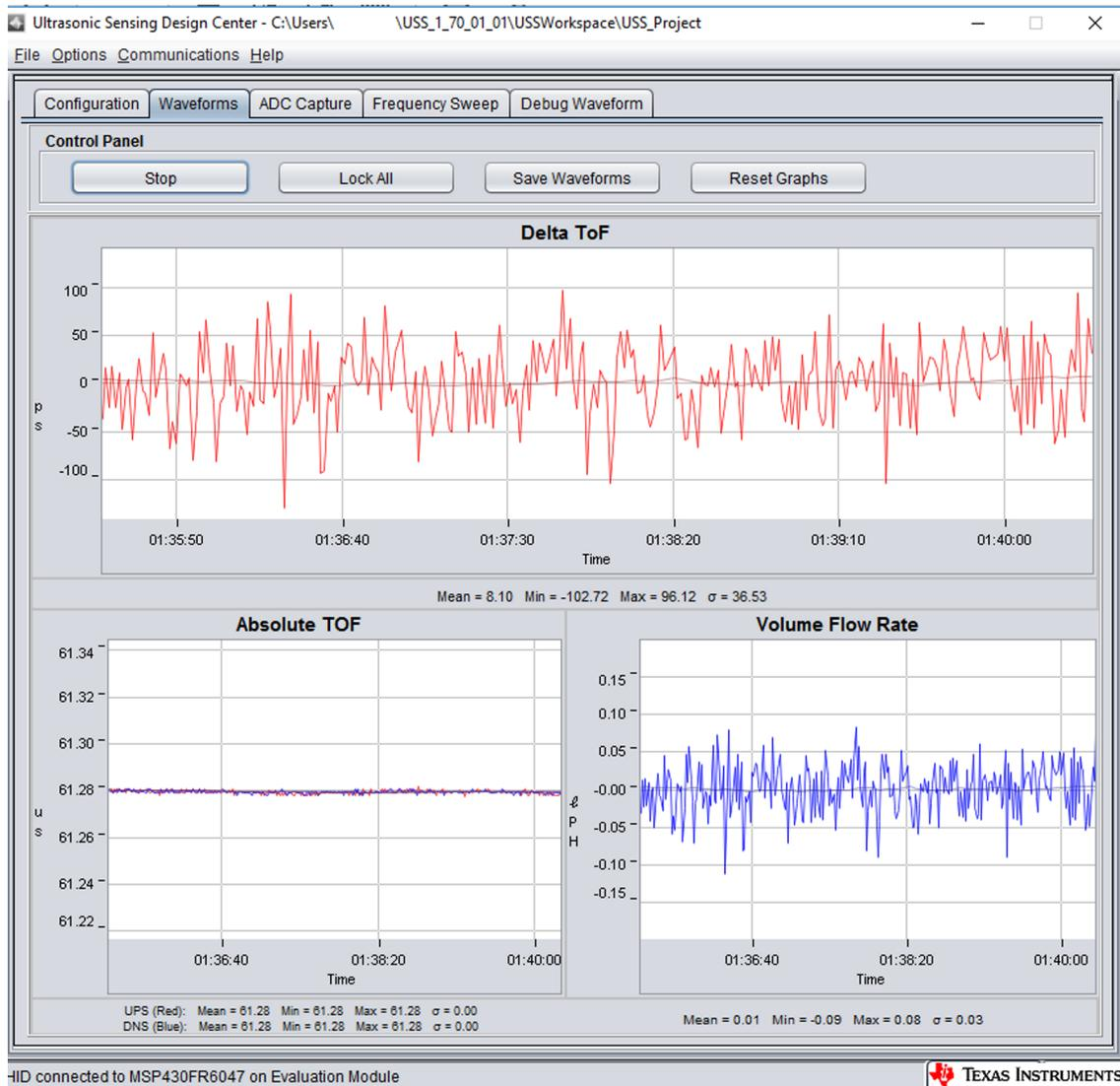
图 12. USS Design Center GUI Waveforms Window
