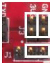
图 6. USB (eZ-FET) Power Jumper Configuration
