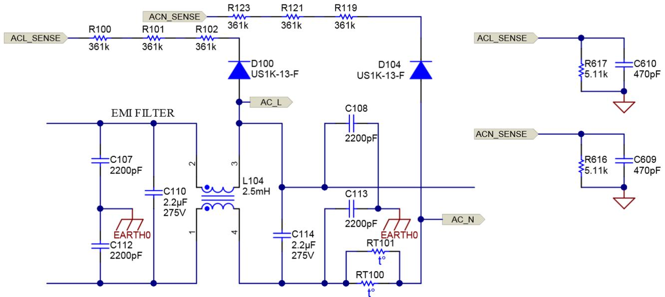
图 14. Schematic of Voltage Dividers for AC Input Voltage Sense
