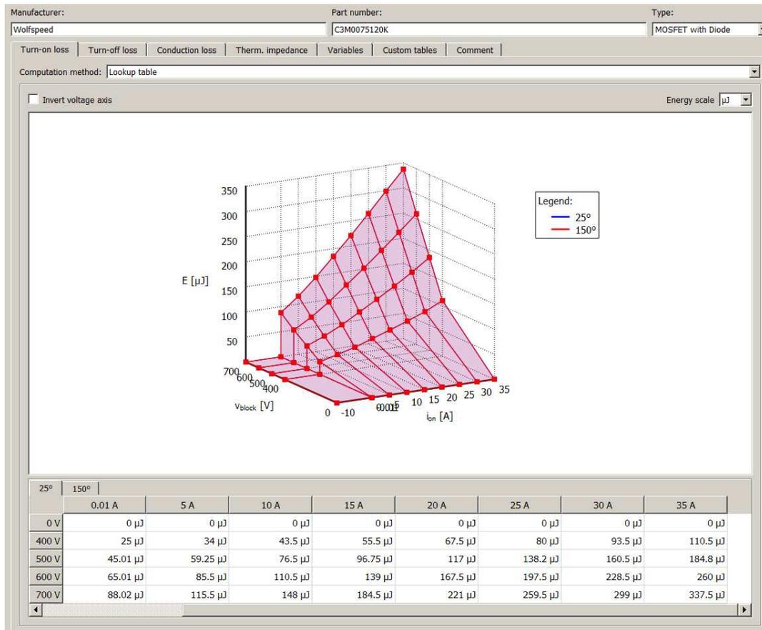
图 10. PLECS® Simulation Model for Power Losses
