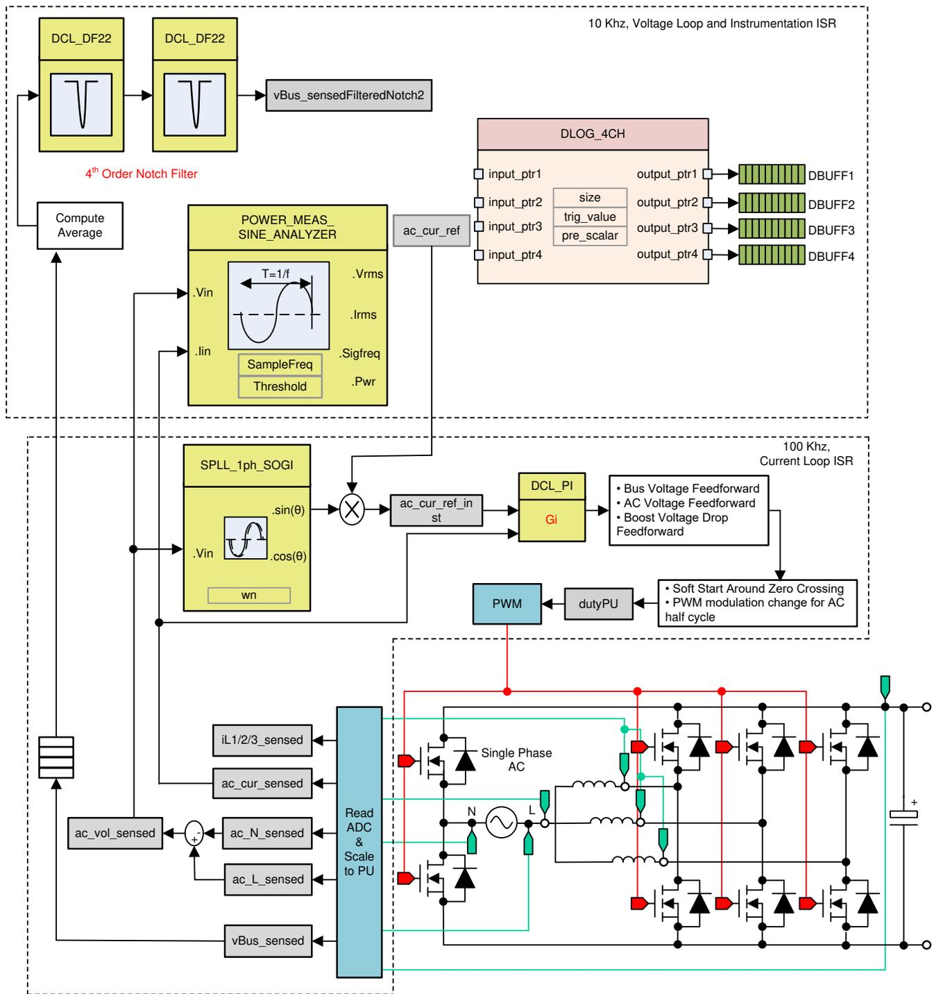
图 31. Build Level 2 Control Software Diagram: Closed Current Loop AC
