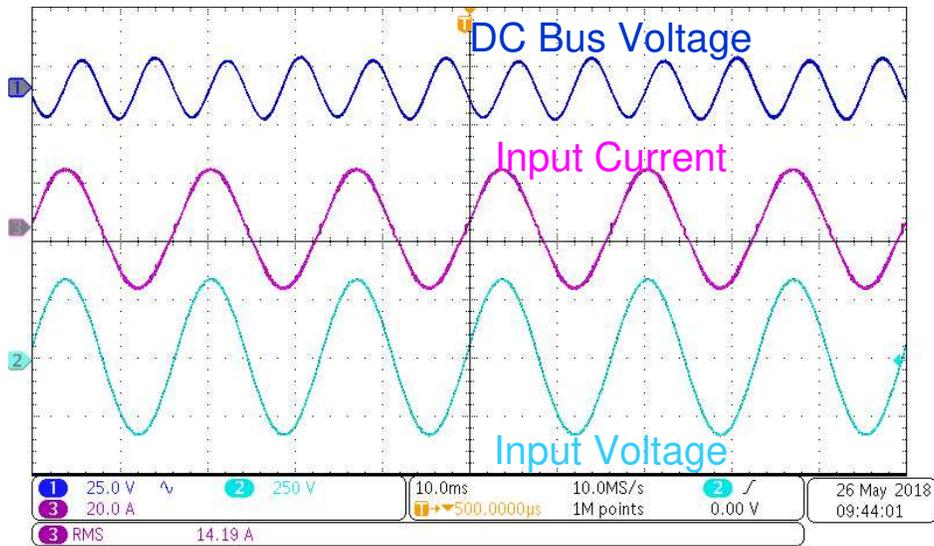
图 63. Steady State Waveforms at 240-V AC Input, 400-V DC Output and 3.3-kW Load
