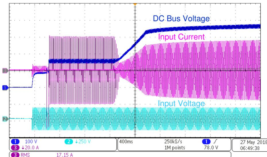
图 47. Startup at 120-V AC Input, 400-V DC Output and 3.3-kW Load
