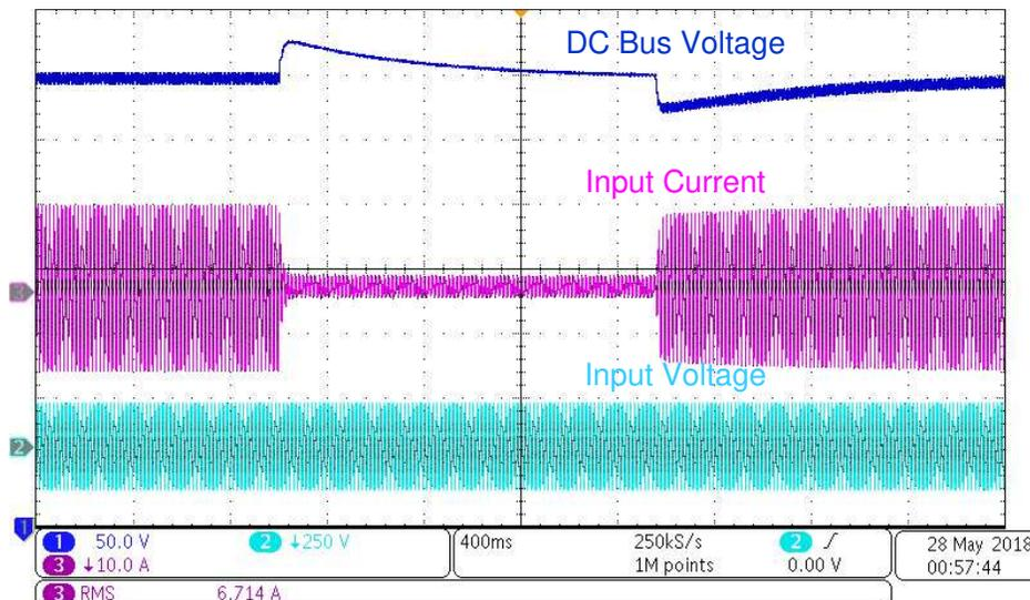
图 44. Voltage Transient Without Non-Linear Voltage Loop,  $V_{in}$  120 V<sub>rms</sub>, 1-kW to 100-W Transient, Overshoot 26 V
