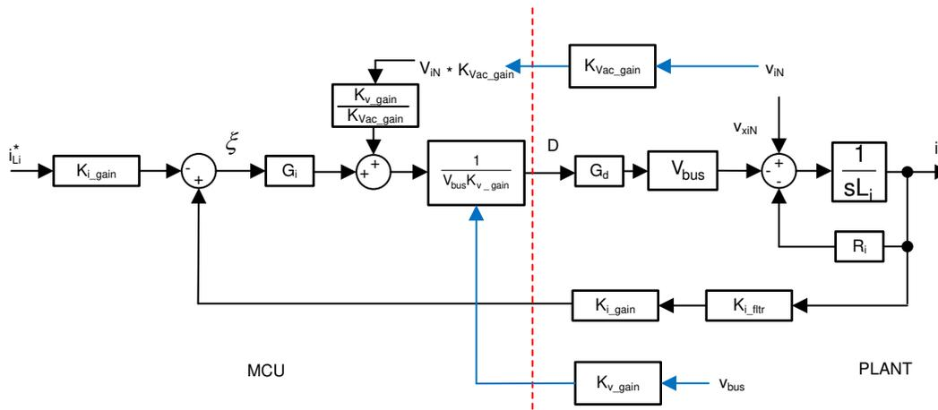
图 7. Current Loop Control Model
