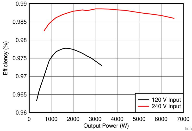
图 70. Efficiency Comparison at 120-V and 240-V Input With Varying Load Conditions
