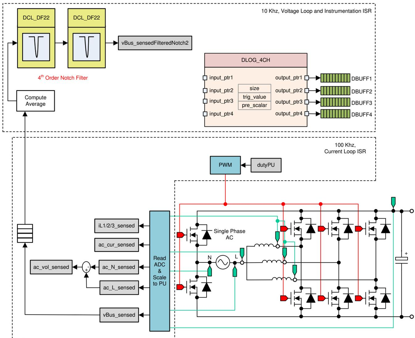
图 23. Build Level 1 Control Software Diagram: Open Loop Project
