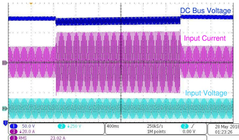
图 55. Load Transient Response From 1.6-kW to 3.3-kW Step With 120-V AC Input
