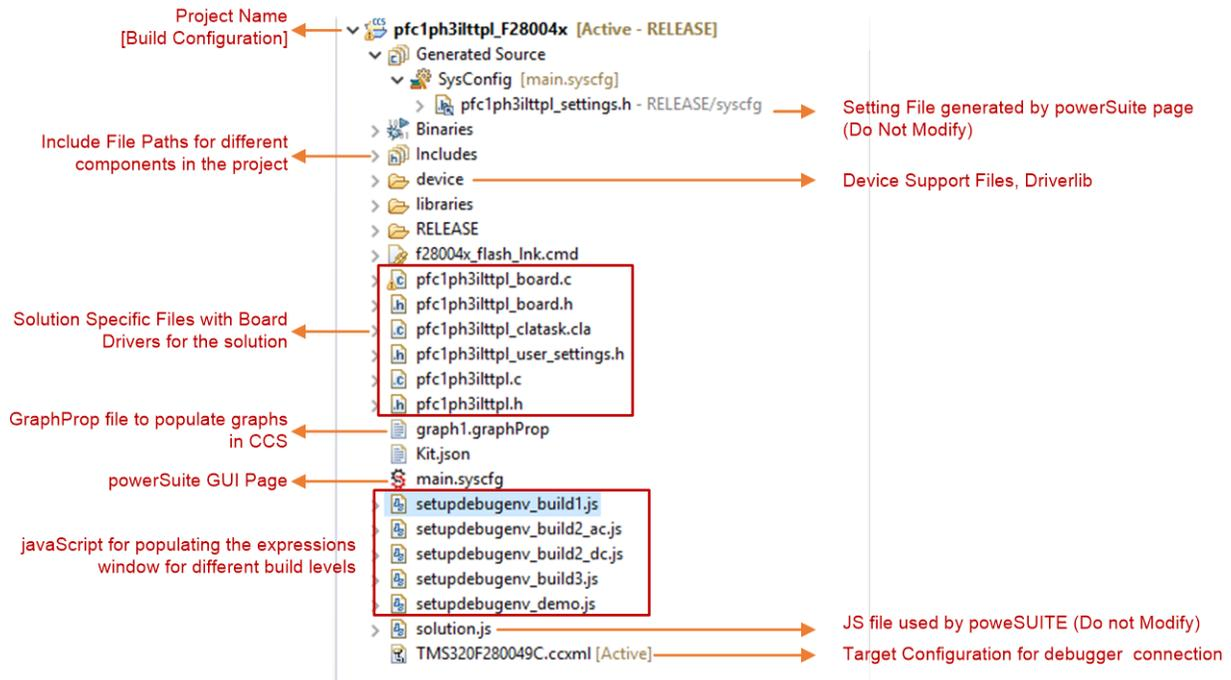
图 20. Project Explorer View of Solution Project
