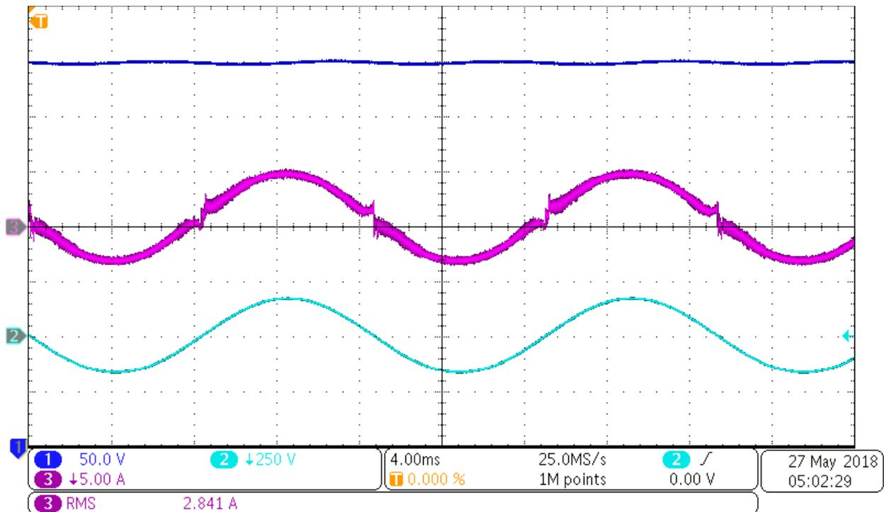
图 34. Input AC Current and Output DC Voltage Waveform
