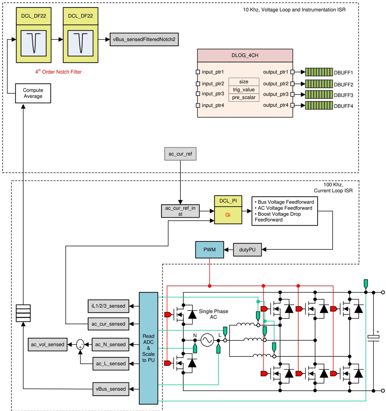
图 26. Build Level 2 Control Software Diagram: Closed Current Loop
