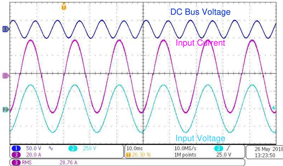
图 65. Steady State Waveforms at 240-V AC Input, 400-V DC Output and 6.6-kW Load
