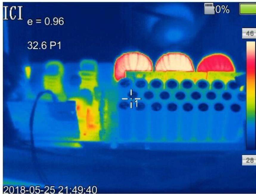
图 75. Thermal Image of the TIDA-01604 at 240-V AC Input With 3.3-kW Load
