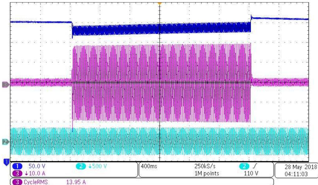
图 67. Load Transient Response From 300-W to 3.3-kW Step With 240-V AC Input
