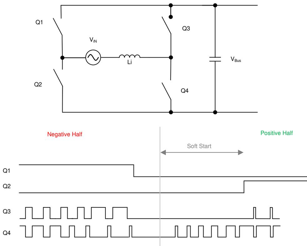
图 9. PWM Sequence With Soft Starting to Reduce Current Spike at Zero-Crossing
