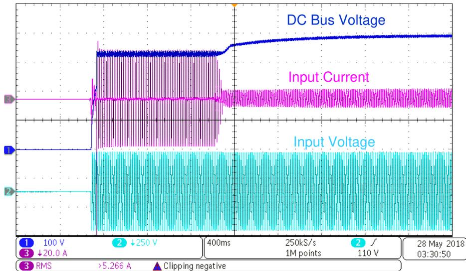
图 60. Startup at 240-V AC Input, 400-V DC Output and 1.6-kW Load
