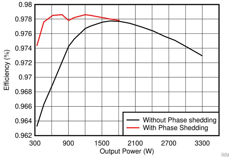
图 59. Efficiency Comparison at 120-V Input With and Without Phase Shedding
