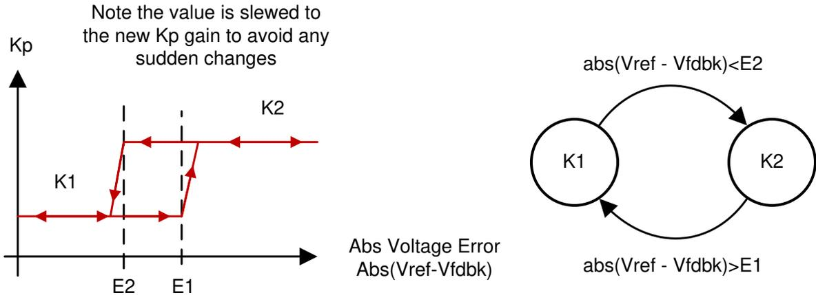
图 43. Non-Linear Voltage Loop With Hysteresis
