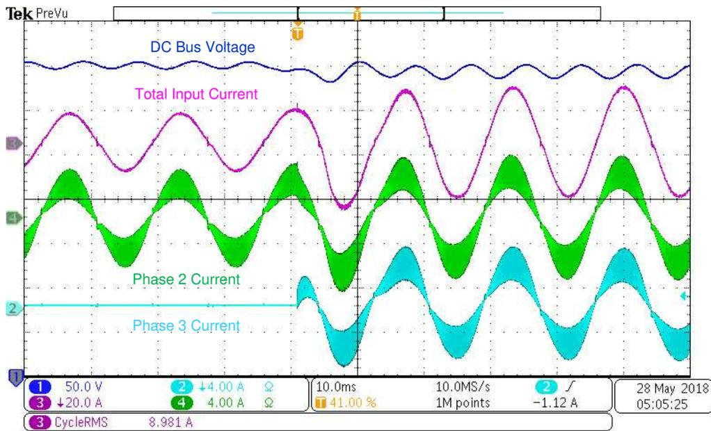
图 58. Phase Added Transition From Dual Phases to Three Phases, Load Step From 720 W to 1.8 kW
