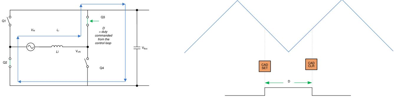
图 6. Single-Phase Diagram of TTPL PFC
