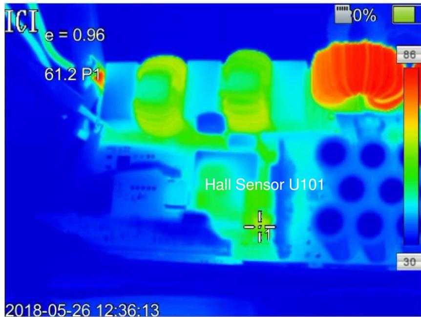
图 74. Thermal Image of the TIDA-01604 at 120-V AC Input With 3.3-kW Load (Focus on the Hall Sensor)
