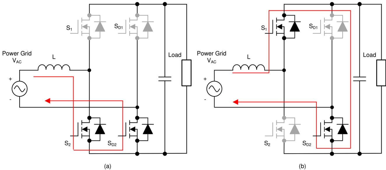
图 2. Totem-Pole Bridgeless PFC Operation During Positive Half Cycle:
