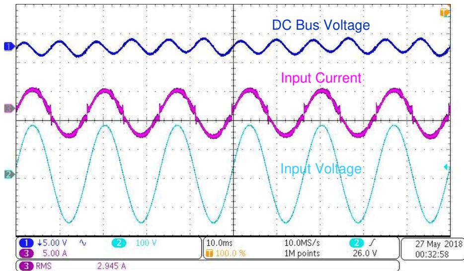
图 49. Steady State Waveforms at 120-V AC Input, 400-V DC Output and 330-W Load
