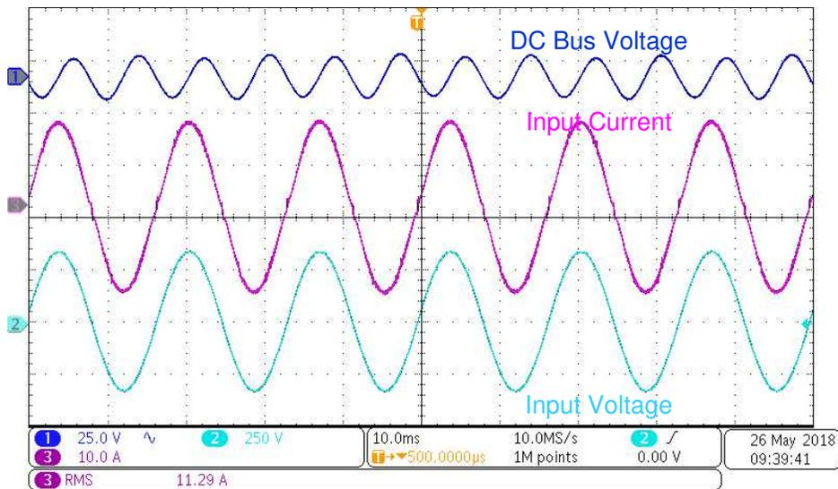
图 62. Steady State Waveforms at 240-V AC Input, 400-V DC Output and 2.6-kW Load
