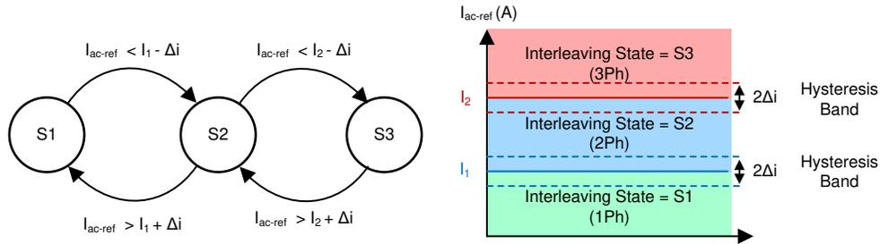
图 41. State Machine for Phase Shedding Control
