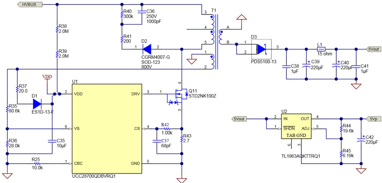
图 11. Schematic of the Auxiliary Power Supply
