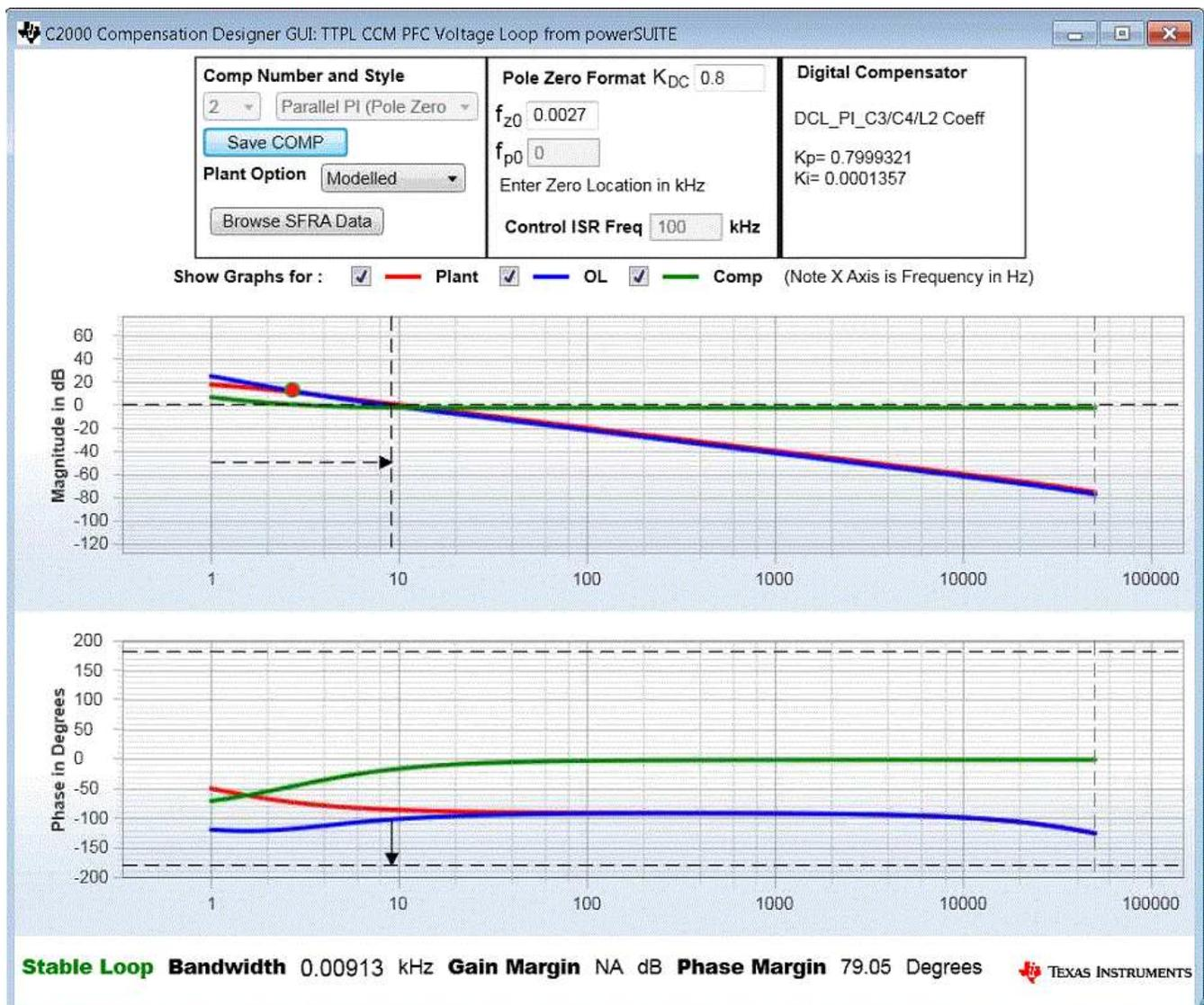
图 36. Voltage Loop Design Using Compensation Designer
