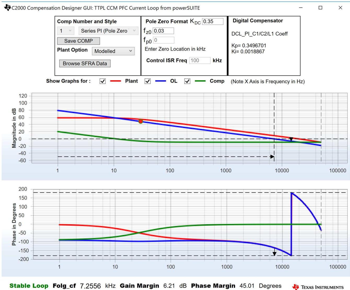
图 27. Current Loop Design Using Compensation Designer
