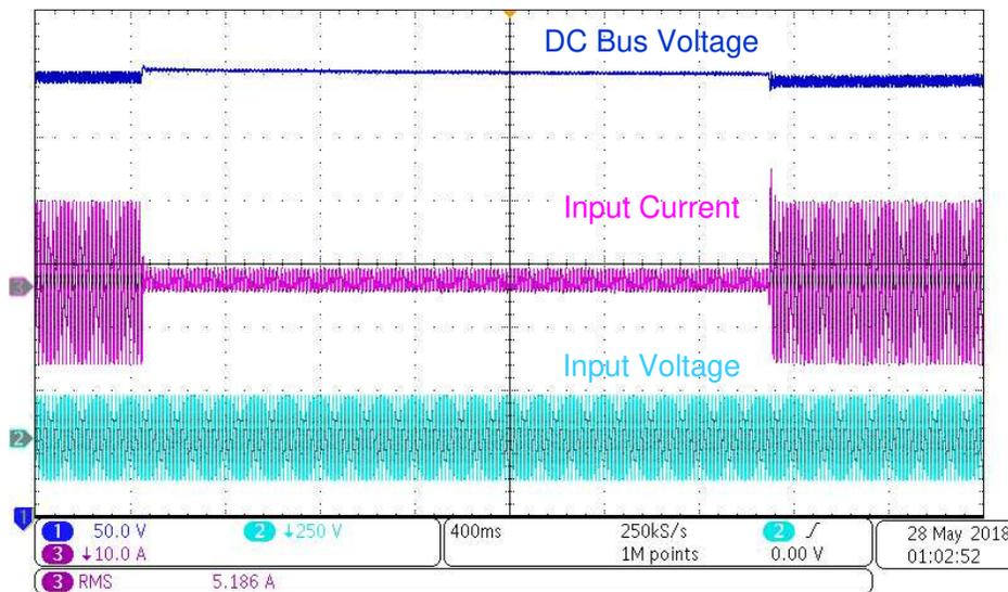
图 45. Voltage Transient With Non-Linear Voltage Loop,  $V_{in}$  120 V<sub>rms</sub>, 1-kW to 100-W Transient, Overshoot 10 V
