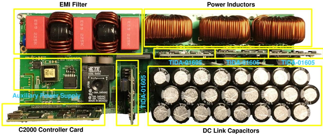
图 16. TIDA-01604 PCB Board—Top View
