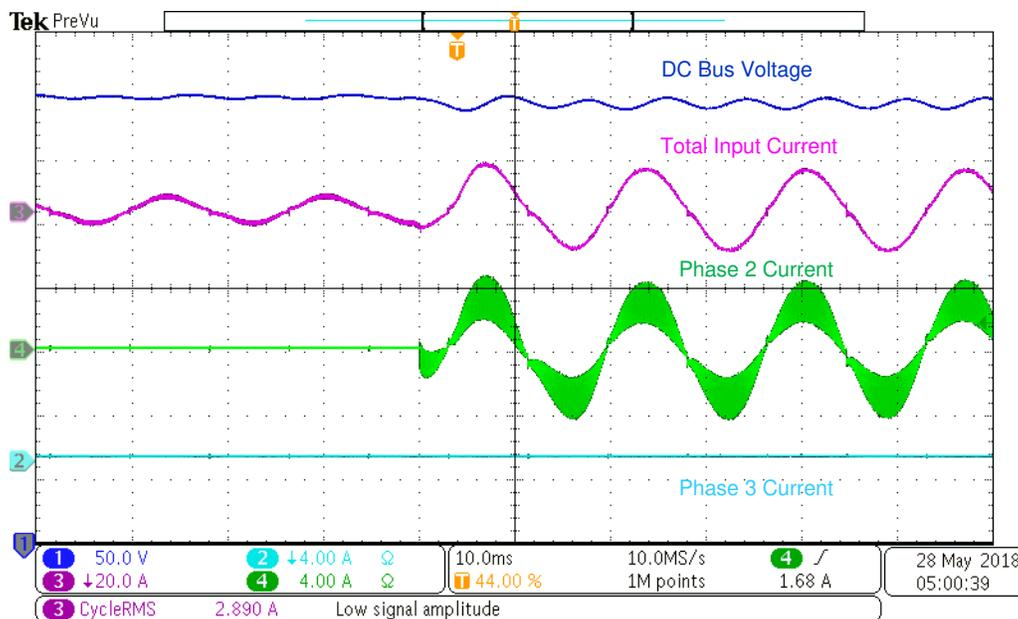
图 56. Phase Added Transition From Single Phase to Dual Phases, Load Step From 320 W to 1 kW
