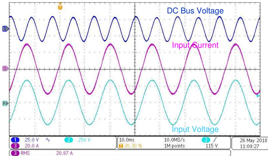
图 64. Steady State Waveforms at 240-V AC Input, 400-V DC Output and 4.8-kW Load
