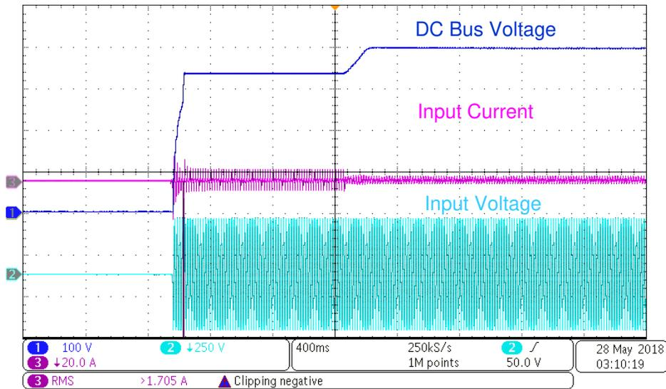
图 61. Startup at 240-V AC Input, 400-V DC Output and No Load
