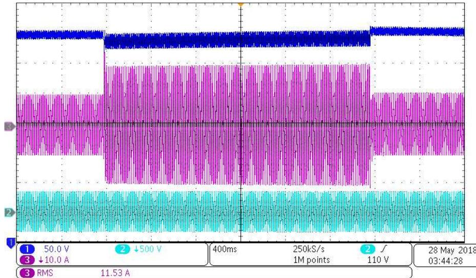
图 66. Load Transient Response From 1.6-kW to 3.3-kW Step With 240-V AC Input
