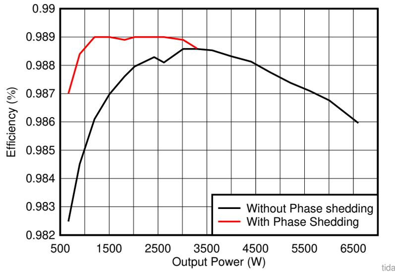
图 69. Efficiency Comparison at 240-V Input With and Without Phase Shedding
