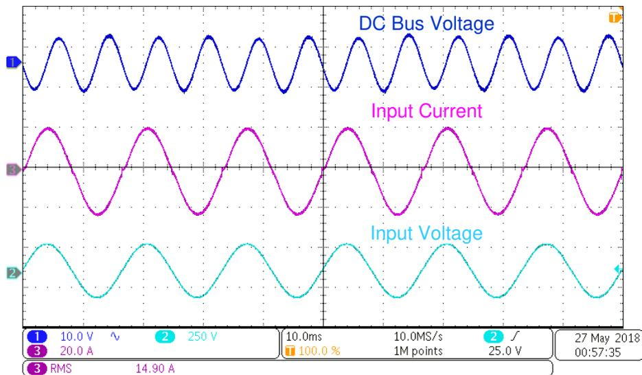
图 50. Steady State Waveforms at 120-V AC Input, 400-V DC Output and 1.65-kW Load
