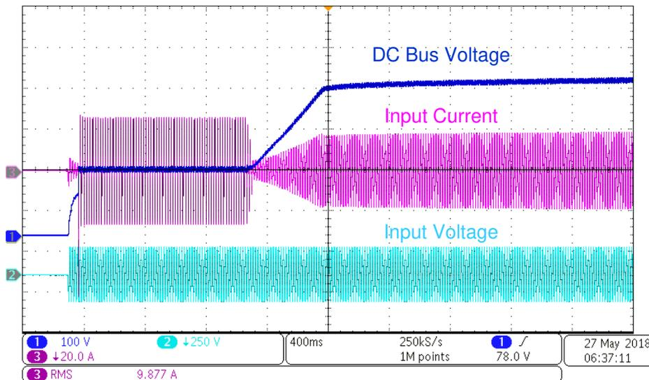
图 46. Startup at 120-V AC Input, 400-V DC Output and 1.6-kW Load
