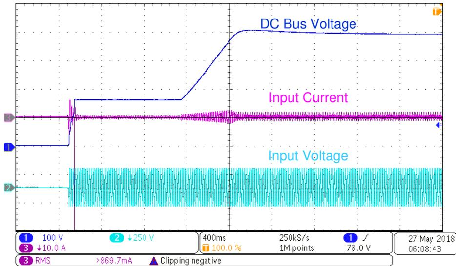
图 48. Startup at 120-V AC Input, 400-V DC Output and No Load
