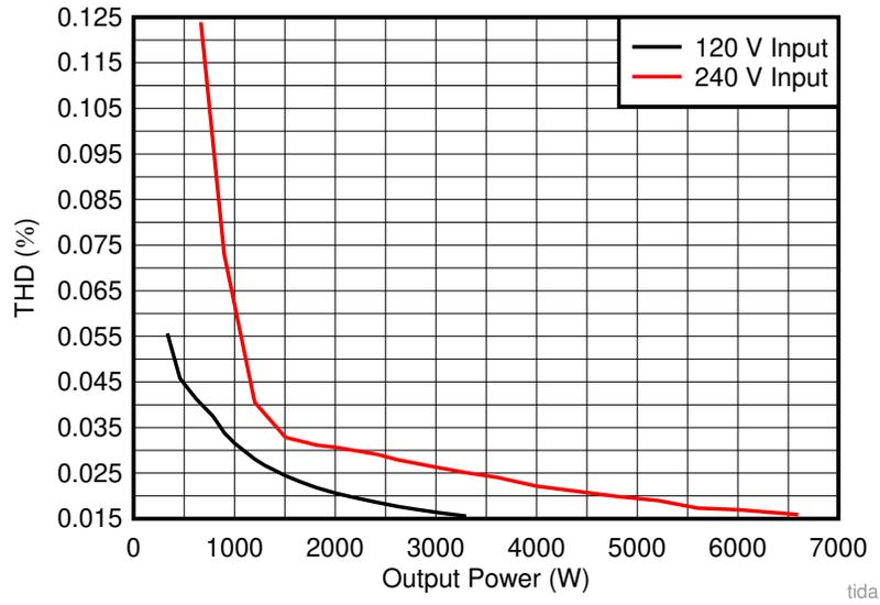
图 72. THD Comparison at 120-V and 240-V Input With Varying Load Conditions
