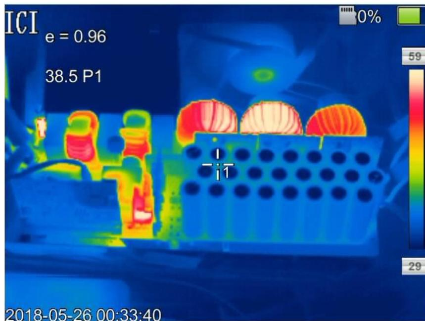
图 76. Thermal Image of the TIDA-01604 at 240-V AC Input With 6.6-kW Load
