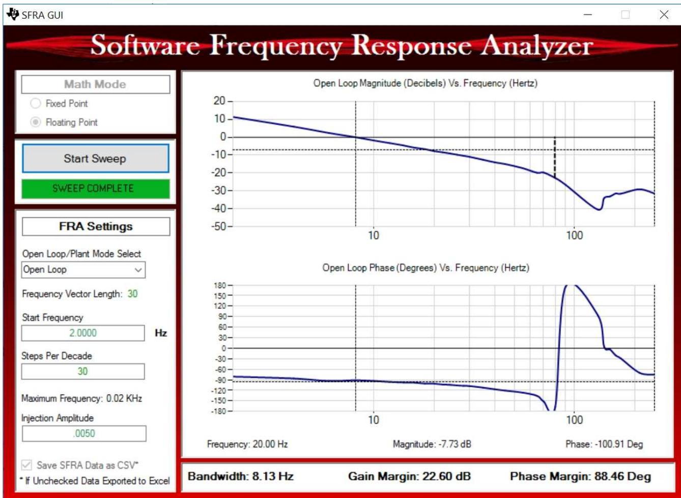
图 39. SFRA Run on Closed Voltage Loop
