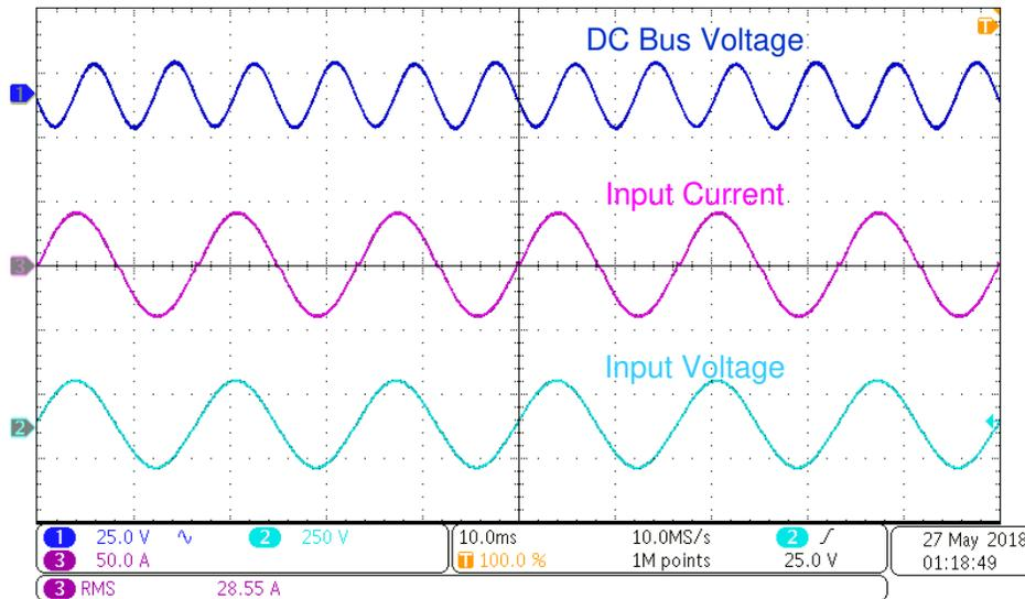
图 52. Steady State Waveforms at 120-V AC Input, 400-V DC Output and 3.3-kW Load
