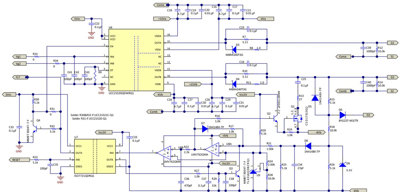
图 15. Schematic of SiC Isolated Gate Driver (TIDA-01605 Design)
