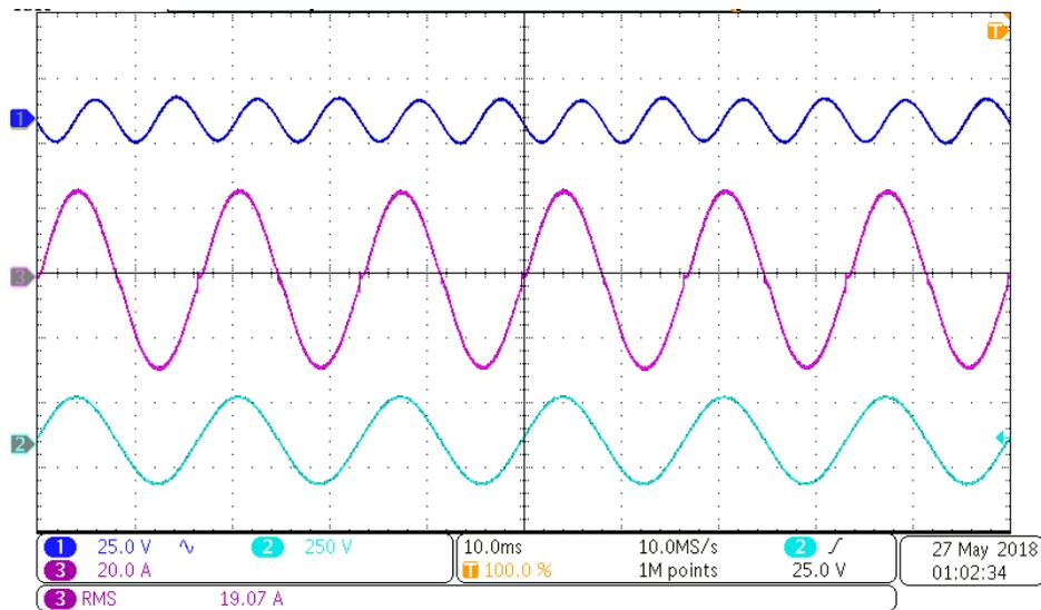
图 51. Steady State Waveforms at 120-V AC Input, 400-V DC Output and 2.2-kW Load
