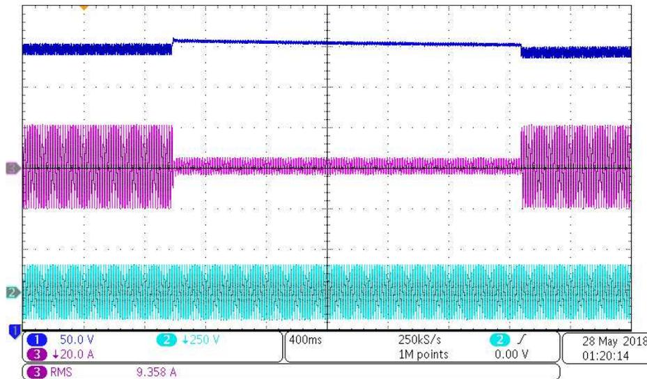
图 53. Load Transient Response From 100-W to 1.6-kW Step With 120-V AC Input
