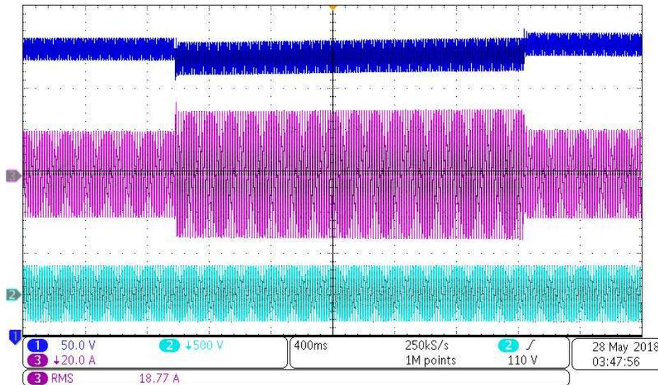
图 68. Load Transient Response From 3.3-kW to 5.5-kW Step With 240-V AC Input
