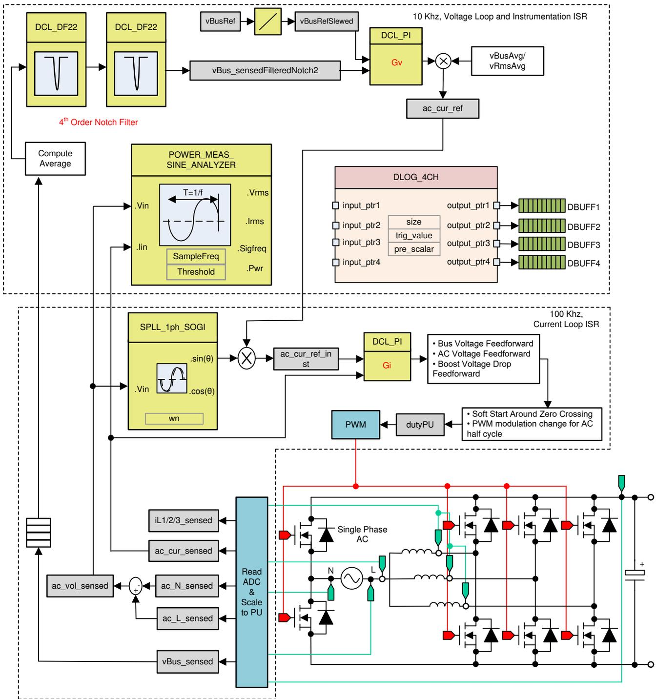
图 35. Build Level 3 Control Diagram: Output Voltage Control With Inner Current Loop
