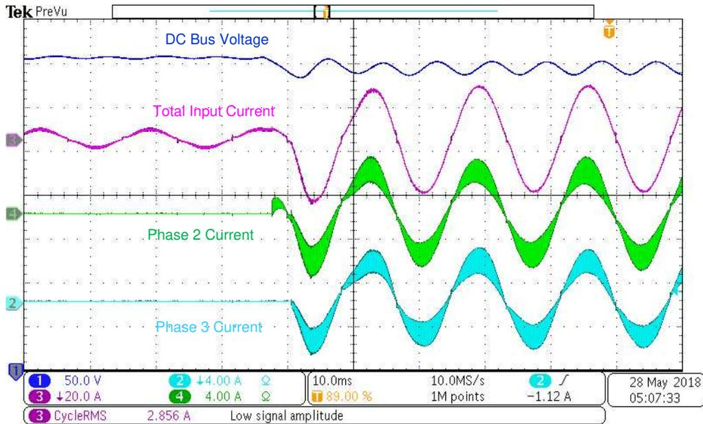
图 57. Phase Added Transition From Single Phase to Three Phases, Load Step From 320 W to 1.8 kW
