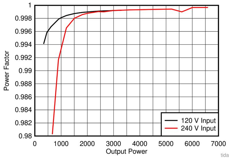
图 71. PF Comparison at 120-V and 240-V Input With Varying Load Conditions
