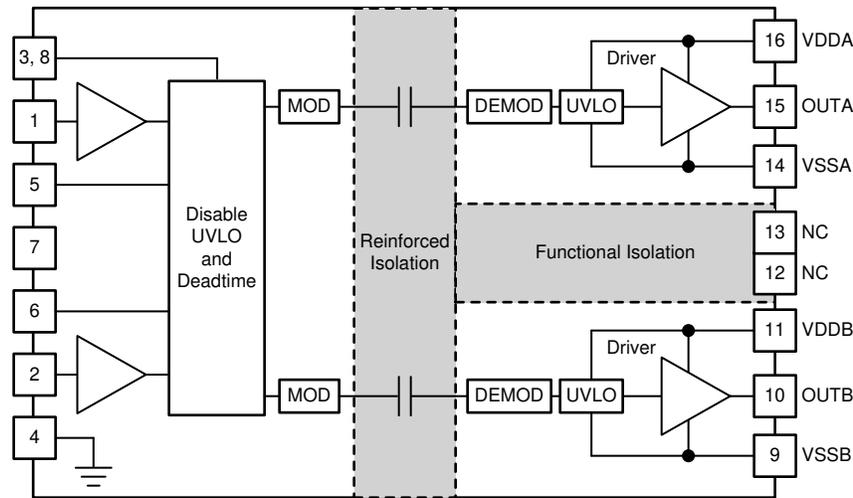
图 5. Functional Block Diagram of UCC21520-Q1
