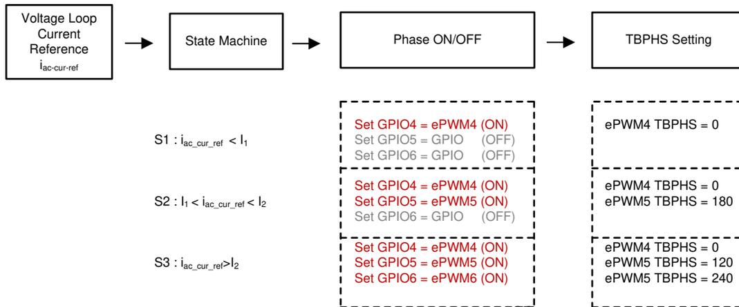
图 42. Implementation of Phase Shedding on TTPL PFC Using C2000™ MCU
