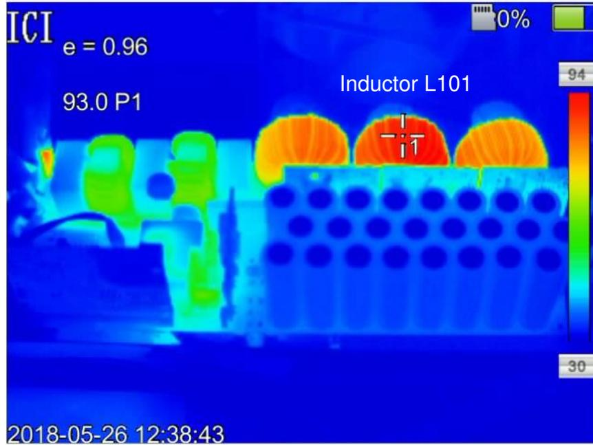
图 73. Thermal Image of the TIDA-01604 at 120-V AC Input With 3.3-kW Load (Focus on the Inductor)
