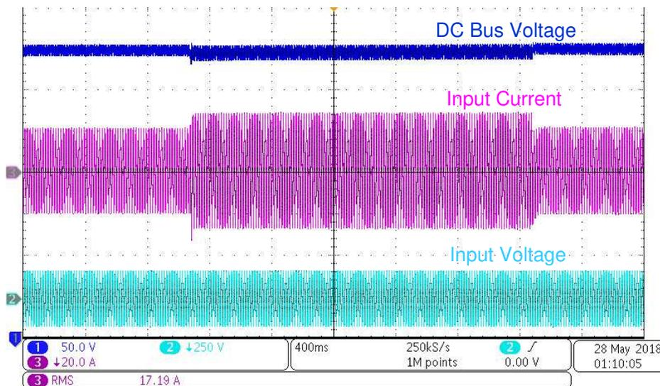
图 54. Load Transient Response From 1.6-kW to 2.2-kW Step With 120-V AC Input
