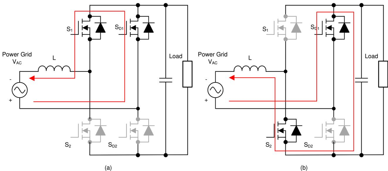
图 3. Totem-Pole Bridgeless PFC Operation During Negative Half Cycle:
