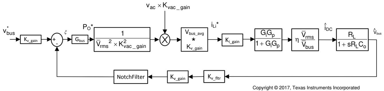
图 8. DC Voltage Loop Control Model
