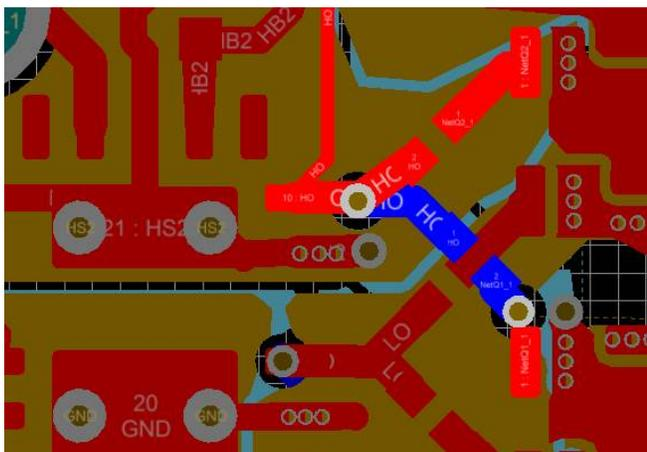
图 4. Gate Drive Path for Paralleled FETs
