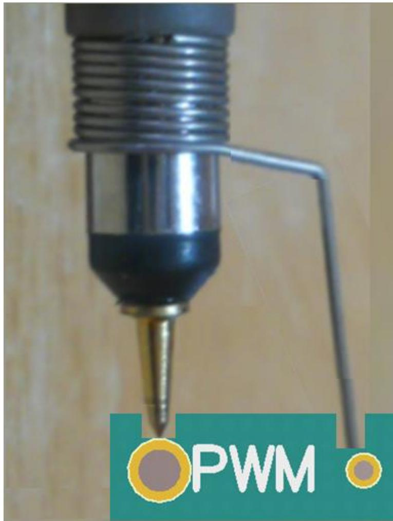
图 9. Low Parasitic Measurement Setup
