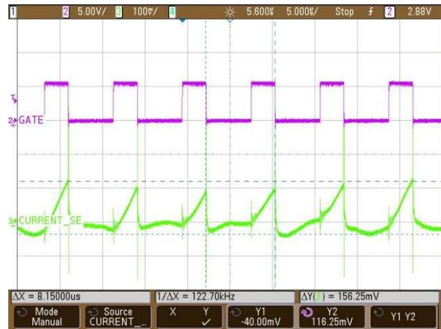
图 22. Current Sense Waveform With Gate Drive at Full Load ( $V_{OUT} = 100\text{ V}$ ,  $I_{OUT} = 125\text{ mA}$ )
