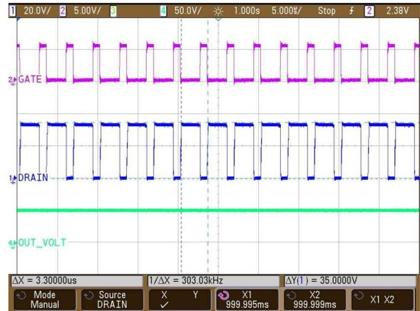
图 63. Gate, Drain, and Output Voltage Waveforms for Synchronization to 300-kHz External Clock
