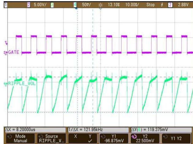
图 31. Output Voltage Ripple at the Negative Rail at 80-V Full Load
