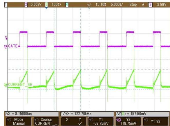
图 36. Current Sense Waveform With Gate Drive at Full Load ( $V_{OUT} = 50\text{ V}$ ， $I_{OUT} = 250\text{ mA}$ )
