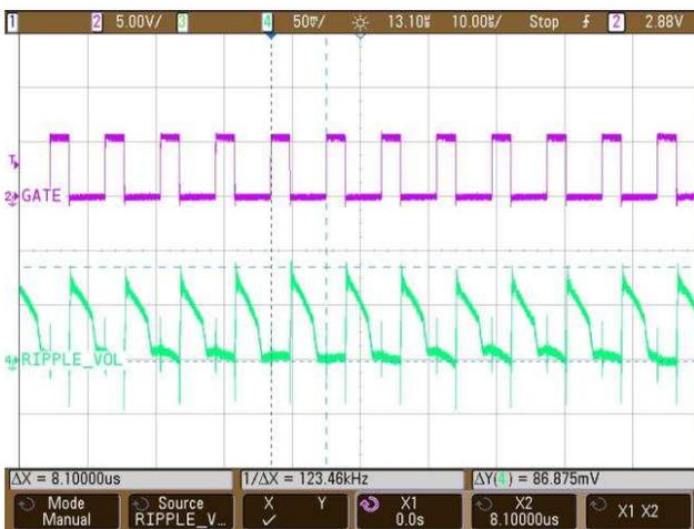
图 23. Output Voltage Ripple at the Positive Rail at 100-V Full Load
