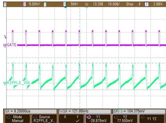
图 45. Output Voltage Ripple at the Negative Rail at 10 V, 300-mA Load
