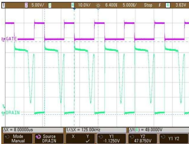
图 21. Stress on the Drain of the MOSFET With Gate Drive at Full Load ( $V_{OUT} = 100\text{ V}$ ,  $I_{OUT} = 125\text{ mA}$ )
