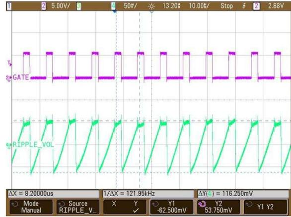
图 38. Output Voltage Ripple at the Negative Rail at 50-V Full Load
