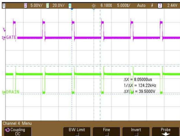
图 42. Stress on the Drain of the MOSFET With Gate Drive at 300-mA Load ( $V_{OUT} = 10\text{ V}$ ,  $I_{OUT} = 300\text{ mA}$ )
