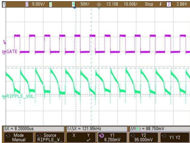
图 30. Output Voltage Ripple at the Positive Rail at 80-V Full Load
