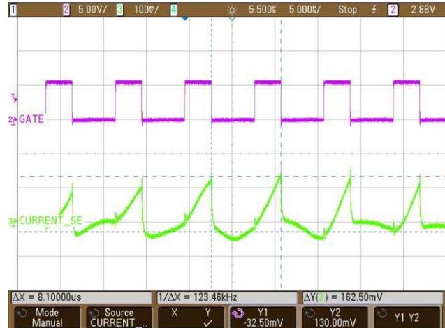
图 29. Current Sense Waveform With Gate Drive at Full Load ( $V_{OUT} = 80\text{ V}$ ,  $I_{OUT} = 160\text{ mA}$ )
