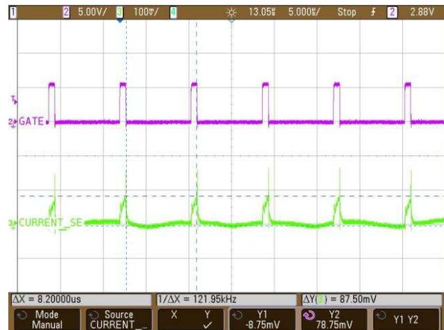
图 43. Current Sense Waveform With Gate Drive at 300-mA Load ( $V_{OUT} = 10\text{ V}$ ,  $I_{OUT} = 300\text{ mA}$ )
