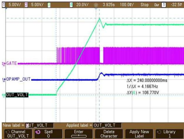
图 58. Soft Start at Set Voltage of 100 V
